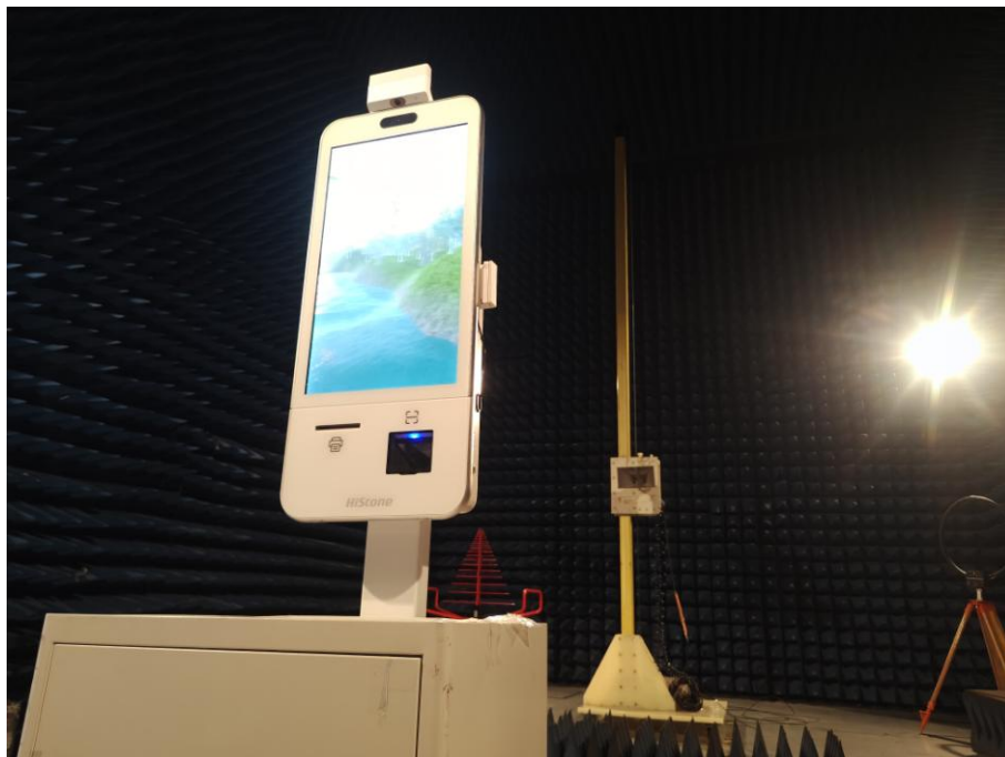
RE TEST SETUP(HS520U+RFID Base)
