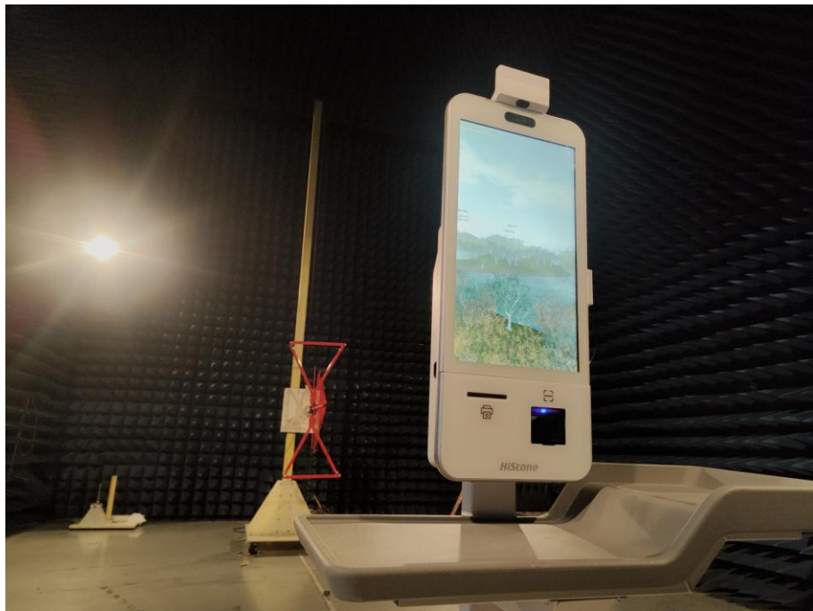
RE TEST SETUP(HS520U)
