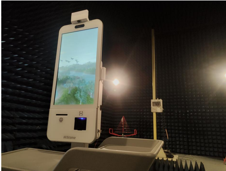
RE TEST SETUP(HS520U)
