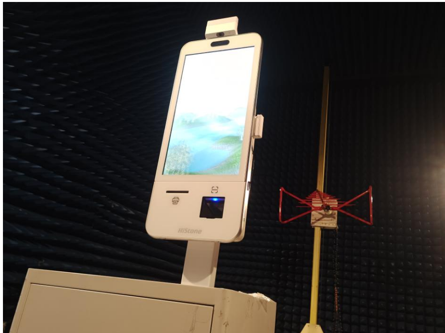
RE TEST SETUP (HS520U+RFID Base)
