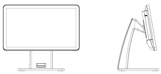
Single screen, length×width×height:  $380 \text{mm}^* 198 \text{mm}^* 327 \text{mm}$ ; main screen flip angle  $0\text{-}45^\circ$
