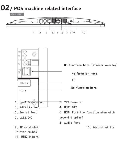
Note 1: This USB interface is only suitable for standard USB devices, such as mouse, keyboard, scanning gun, etc., and the current limit is 500mA.
