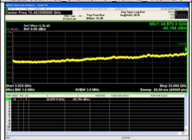
Spurious Emission:5925~25000.0 MHz IEEE 802.11ac Channel 151 40MHz Antenna 0
