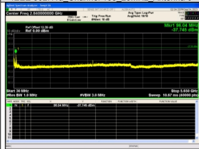
Spurious Emission:30.0~5650 MHz IEEE 802.11n Channel 149 20MHz Antenna 0
