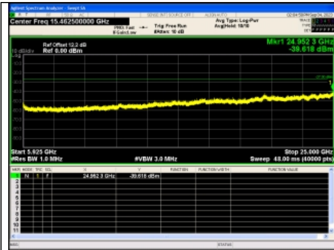
Spurious Emission:5925~25000.0 MHz IEEE 802.11ac Channel 165 20MHz Antenna 0
