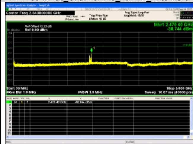
Spurious Emission:30.0~5650 MHz IEEE 802.11ac Channel 157 20MHz Antenna 0
