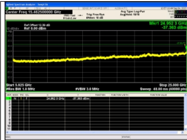
Spurious Emission:5925~25000.0 MHz IEEE 802.11a Channel 149 20MHz Antenna 0
