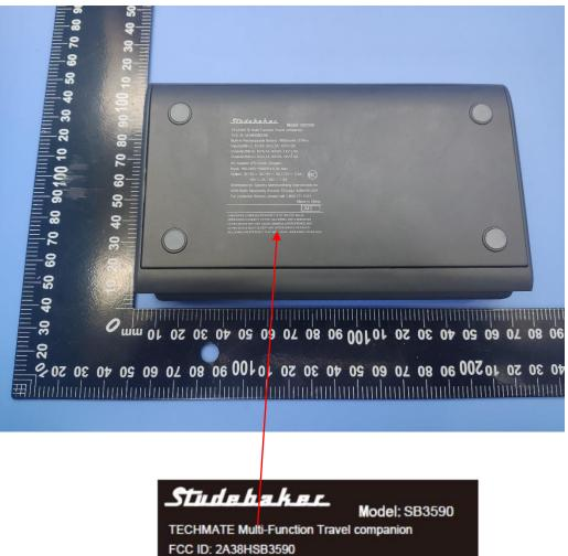
Built-in Rechargeable Battery 10000mAH (37Wh) Input(USB-C): 5V/3A, 9V/2.3A, 12V/1.5A Output(USB-A): 5V/3.1A, 9V/2A, 12V/1.5A Output(USB-C): 5V/3.1A, 9V/2A, 12V/1.5A
