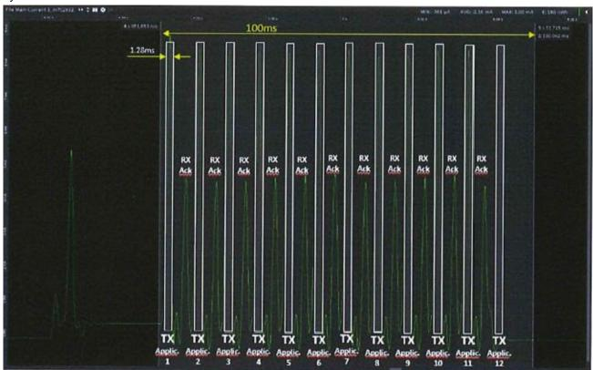
Duty cycle=1.28ms\*12/100ms=15.36% PDCF=20\*LOG(duty cycle)=20\*LOG(15.36%)=-16.27
