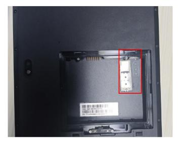
Put the TF card and Nano SIM card back to their right positions as shown in the figure below, then to use.
