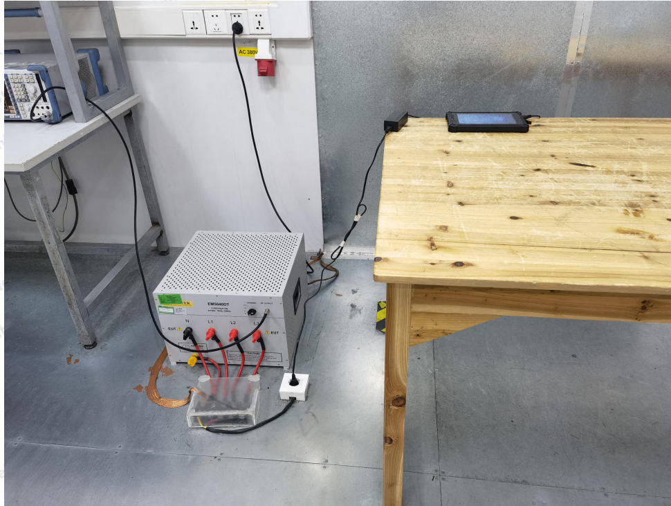
Photo of Conducted Emission Measurement
