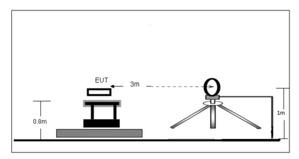
(B) Radiated Emission Test-Up Frequency 30MHz~1GHz
