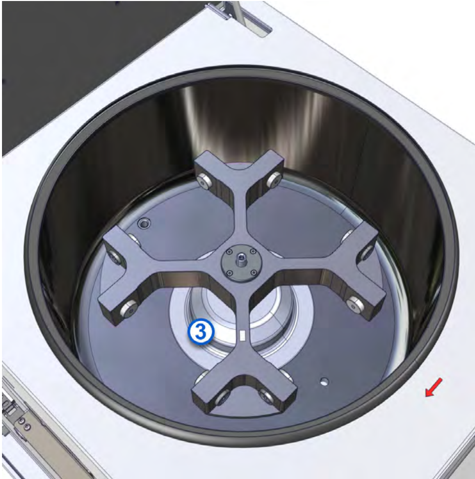
Figure 40: Inspecting motor rubber sleeve
