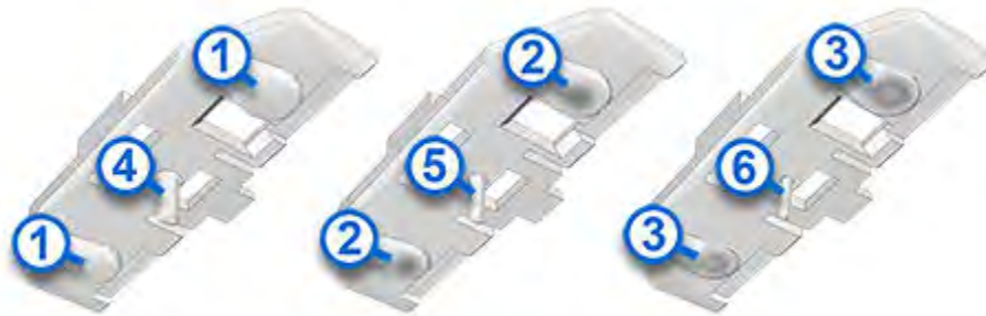
Figure 43: Slider wear on the front underseal of the CAR
