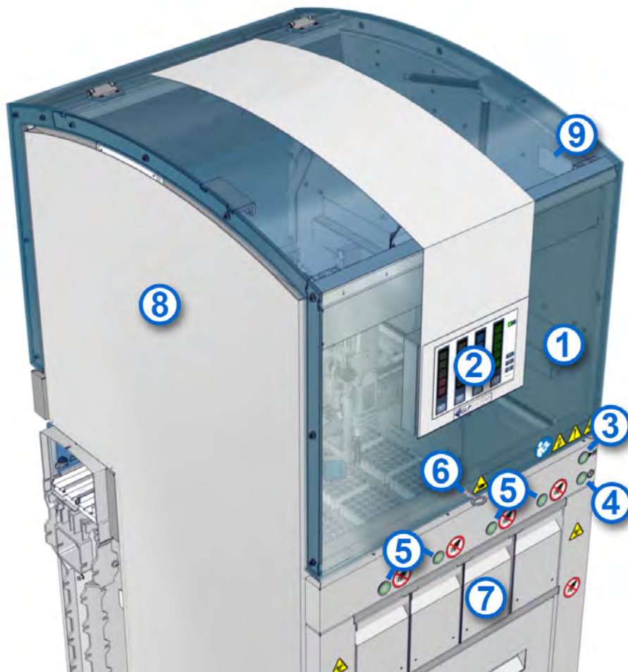
Figure 6: Exterior front view of the IOM
