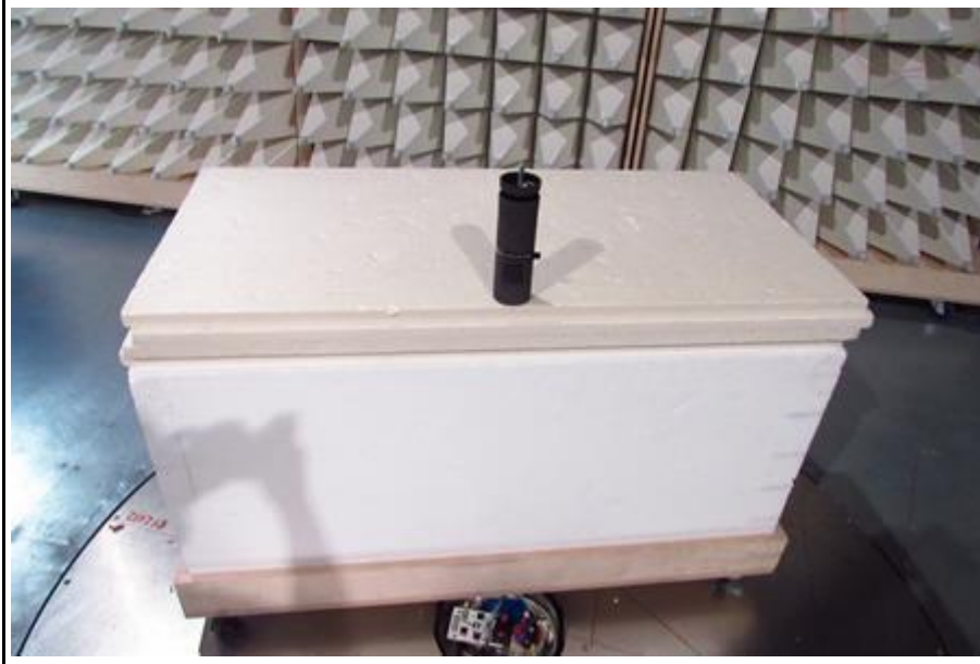
Setup for measurements below 1 GHz
