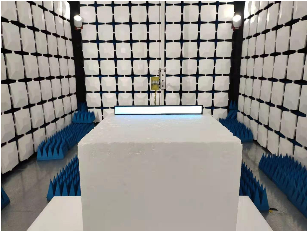
Below 1GHz for radiated emission test setup
