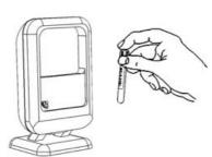
**Scanning a tube** with the barcode reader until the reader emits a "beep".
