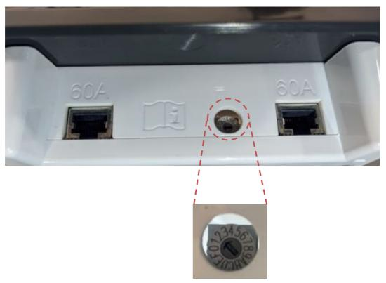
The screw arrow is pointing at number 2. The connection order must be ascendant, as that is how the modules are displayed on Quicklab's main screen.
