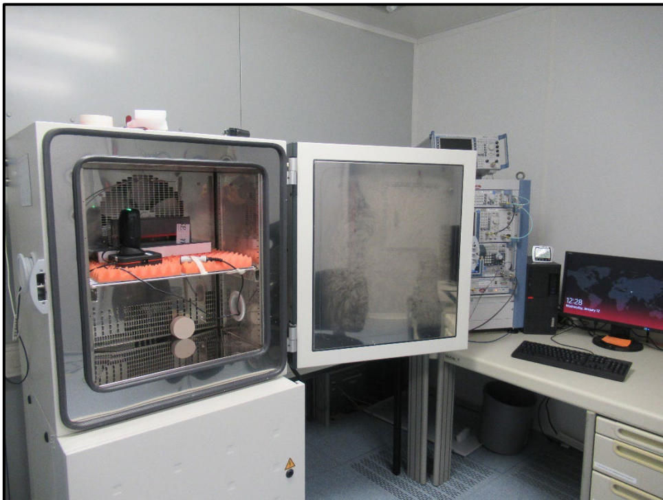
Photo 6 Extreme Temperature Test Setup
