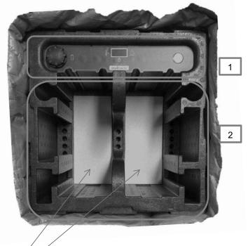
Before starting the cleaning process, please remove the "absorbent pads". If any spilling occurs, they will be destroyed and need to be replaced.
