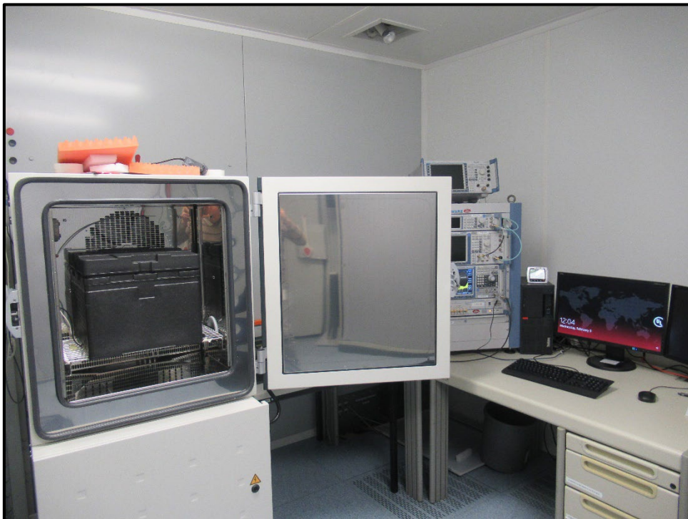
Photo 6 Extreme Temperature Test Setup
