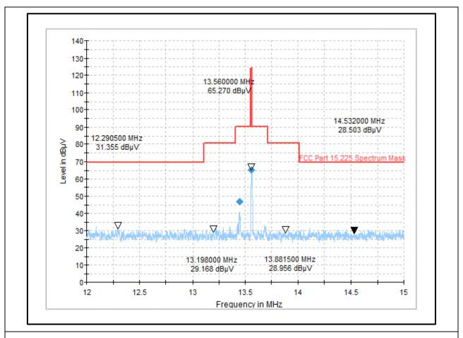
Fundamental field strength and spectrum mask / measured at 3 metres / measured in a semi-anechoic chamber
