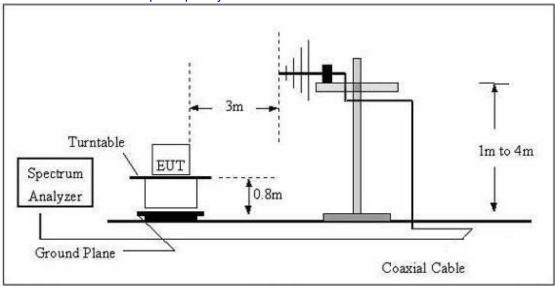
(C) Radiated Emission Test-Up Frequency Above 1GHz
