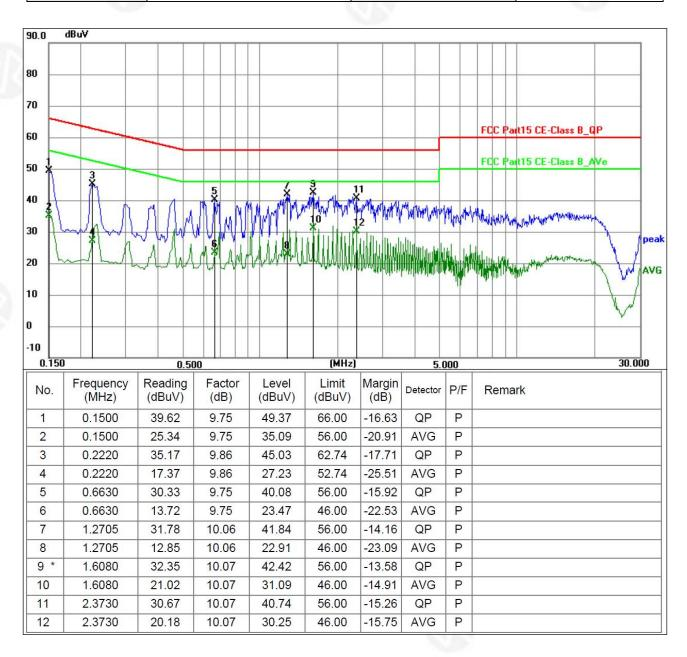
1.An initial pre-scan was performed on the line and neutral lines with peak detector.
