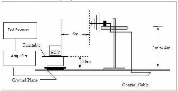
(C) Radiated Emission Test-Up Frequency Above 1GHz
