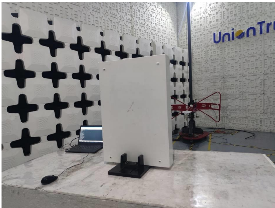
Radiated emission Test Setup (30 MHz~1 GHz)
