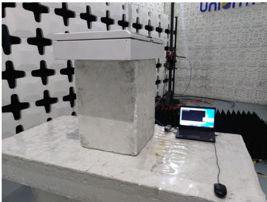
Radiated emission Test Setup (Above 1 GHz)
