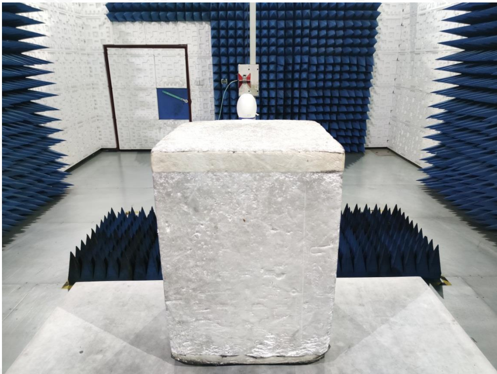
FCC RADIATED EMISSION TEST SETUP ABOVE 1GHZ
