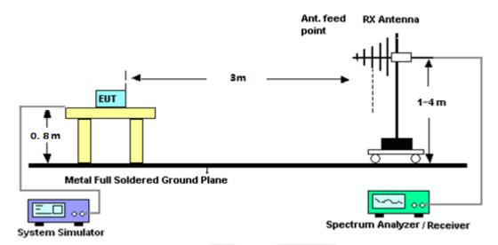
For radiated test from above 1GHz
