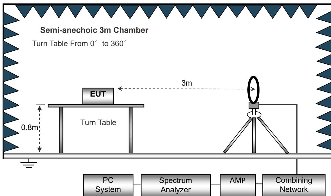
The test setup for emission measurement from 30MHz to 1GHz.
