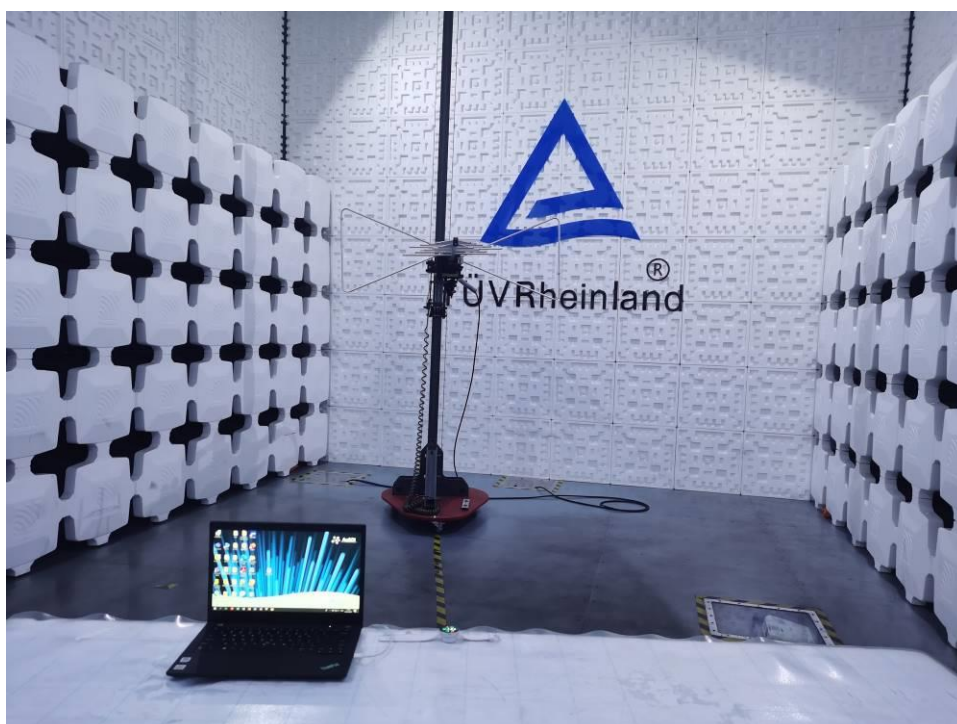
Photograph 4: Set-up photo for Radiated Emission, Below 1GHz
