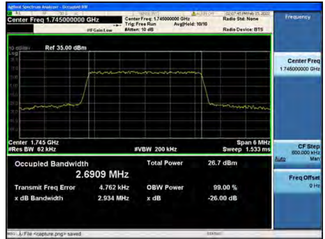
Band66 / 3MHz / High CH / QPSK
