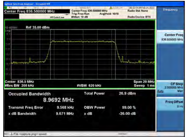
Band26Part22 / 10MHz / High CH / QPSK
