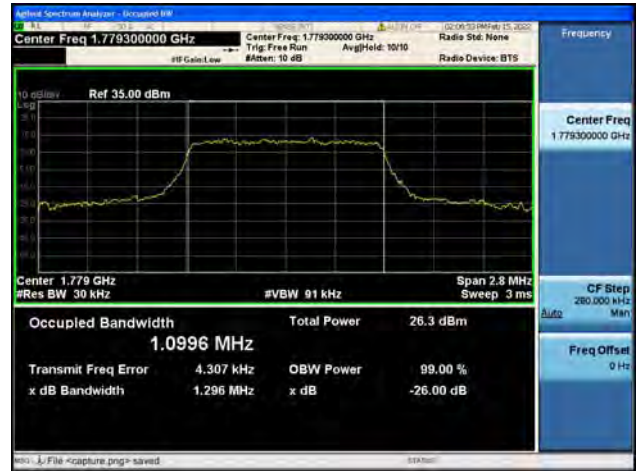
Band66 / 3MHz / Low CH / QPSK
