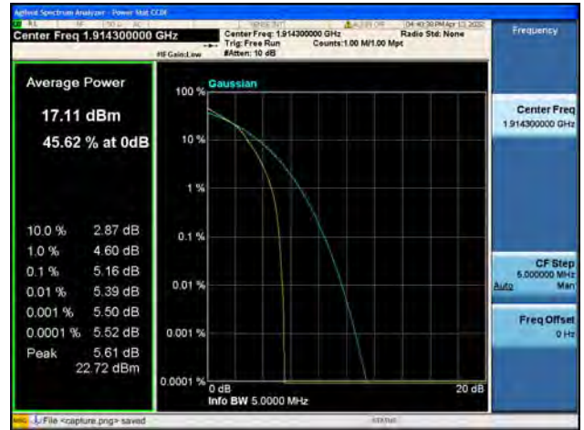
Band25 / 3MHz / Low CH / QPSK
