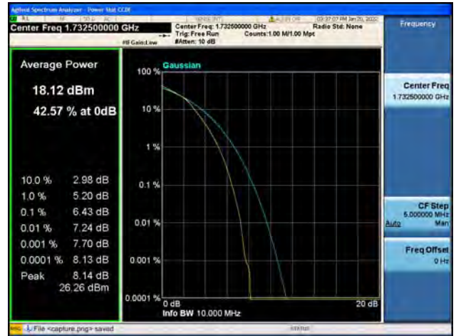
Band4 / 10MHz / High CH / QPSK
