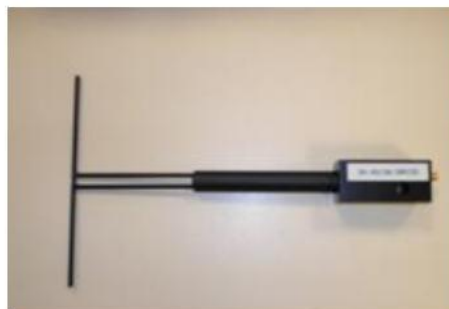
Figure 1 – Satimo COMOSAR Validation Dipole
