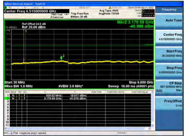
Band26Part22 / 1.4MHz / Mid CH / 16QAM
