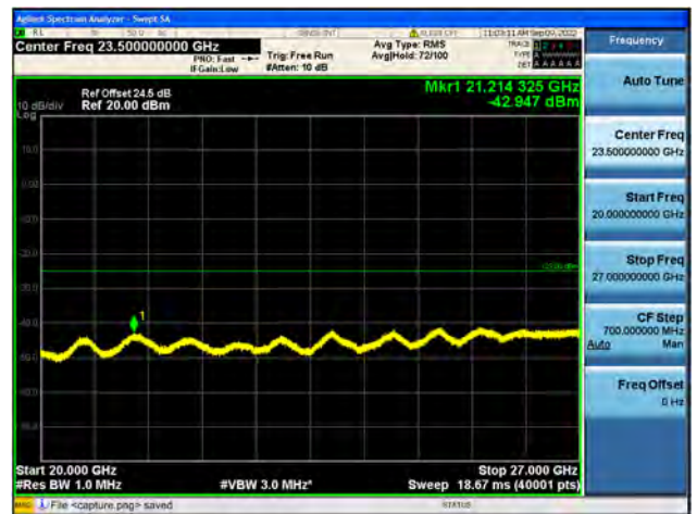
Band41-20G-27G / 15MHz / High CH / 16QAM
