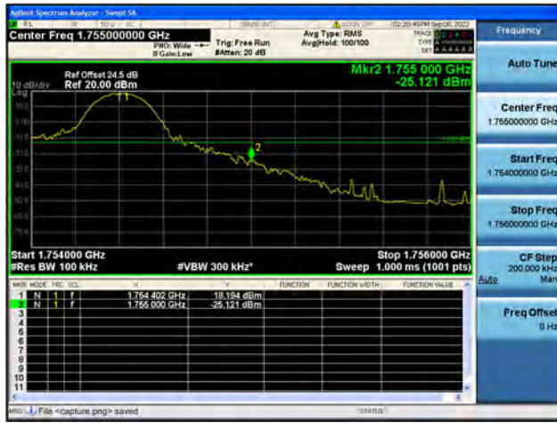
Band4 / 10MHz / High CH / QPSK / 1 RB
