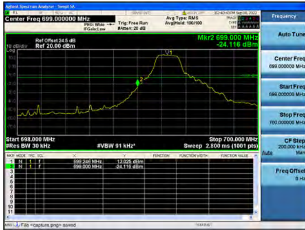
Band12 / 1.4MHz / High CH / QPSK / 1 RB
