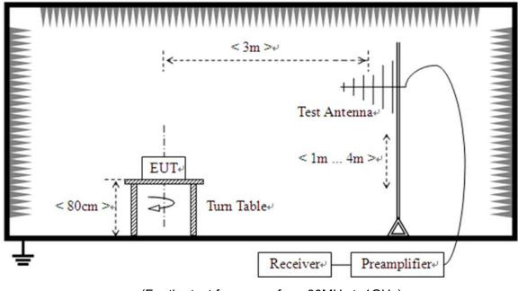
(For the test frequency from 30MHz to1GHz)
