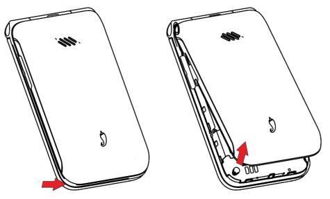
Step 2. Remove the battery using your fingernail to lift from the top.
