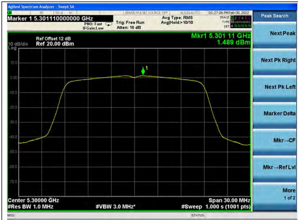
(Channel 60, 5300MHz, 802.11ac (VHT20))
