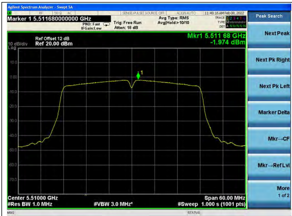
(Channel 102, 5510MHz, 802.11ac (VHT40))
