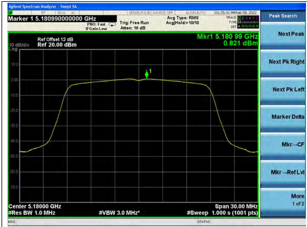
(Channel 36, 5180MHz, 802.11ac (VHT20))
