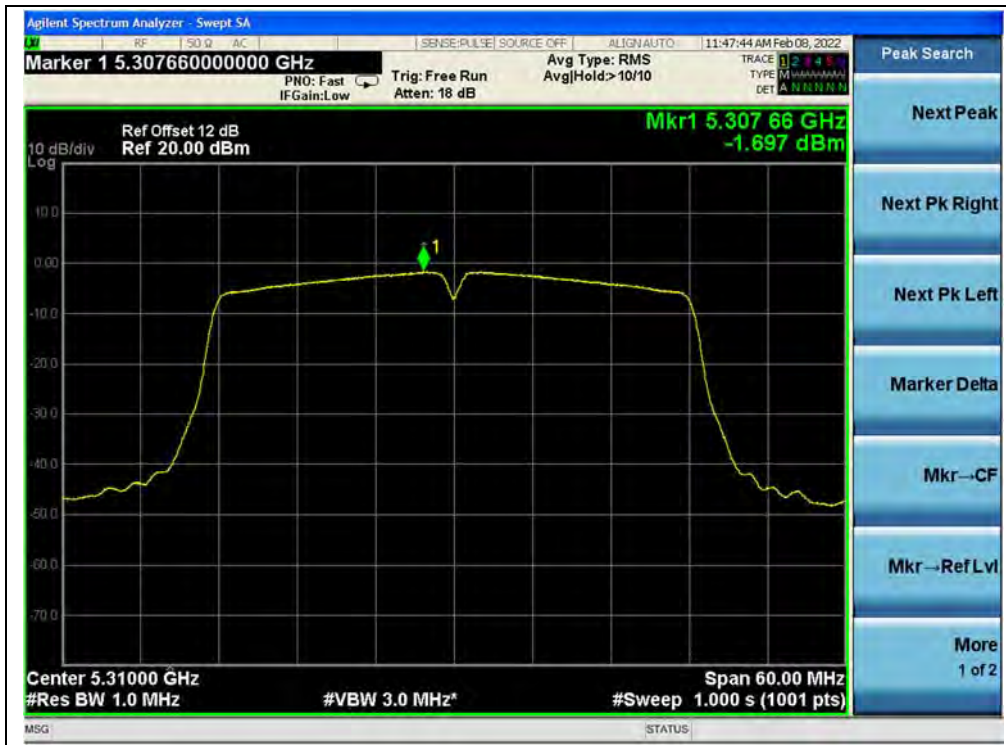
(Channel 62, 5310MHz, 802.11ac (VHT40))
