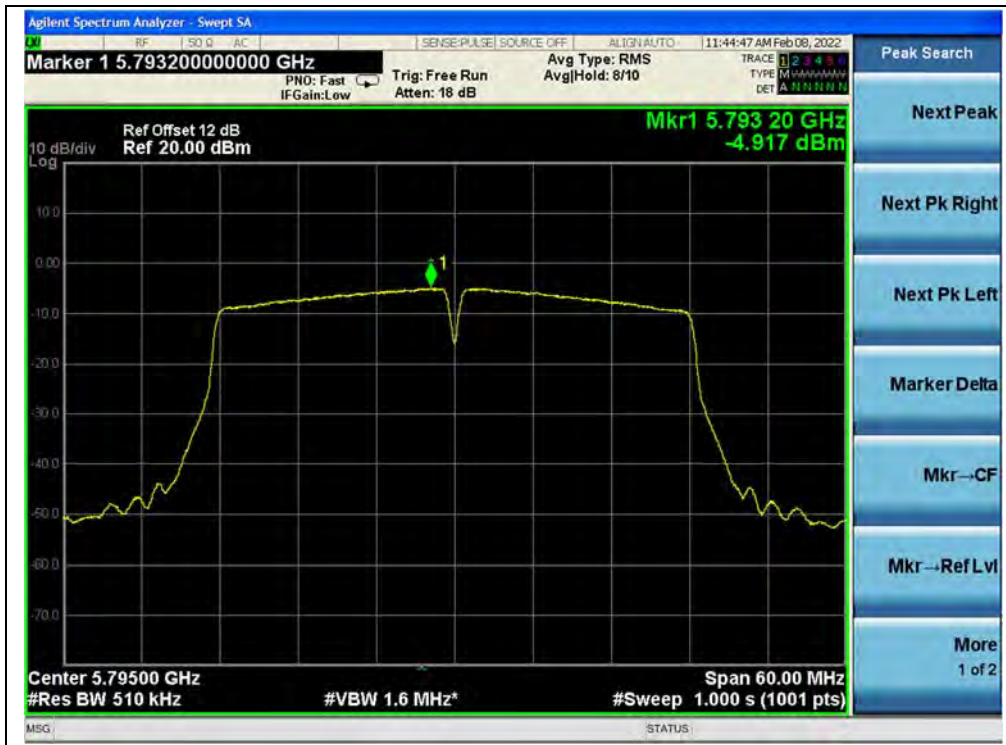
(Channel 159, 5795MHz, 802.11ac (VHT40))
