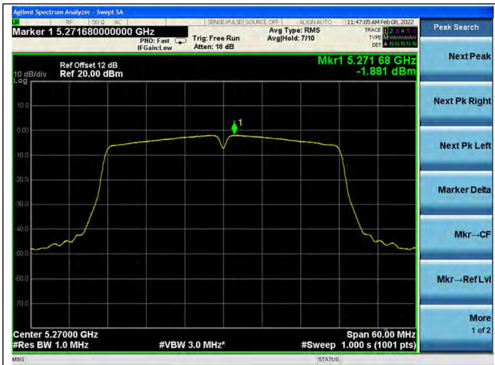
(Channel 54, 5270MHz, 802.11ac (VHT40))
