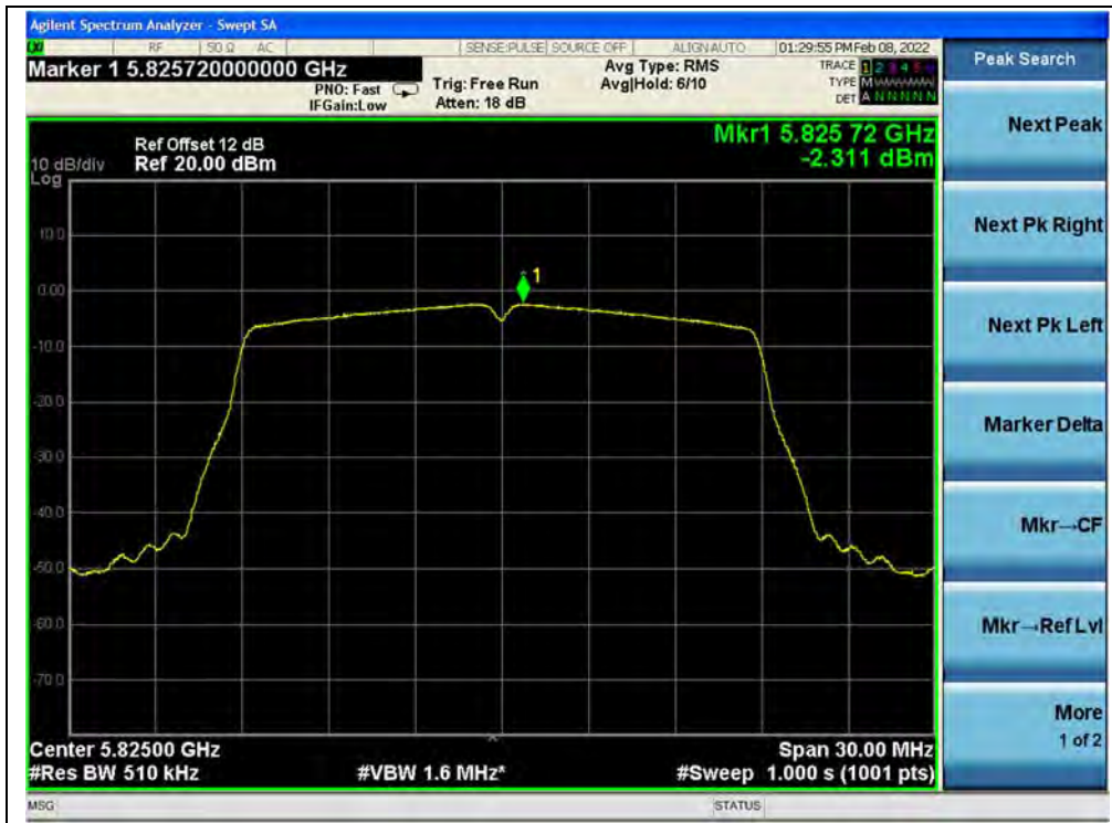
(Channel 165, 5825MHz, 802.11ac (VHT20))
