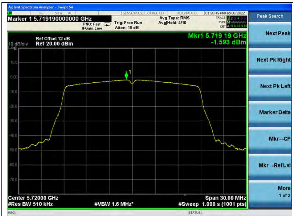
(Channel 144, 5720MHz, 802.11ac(VHT20))
