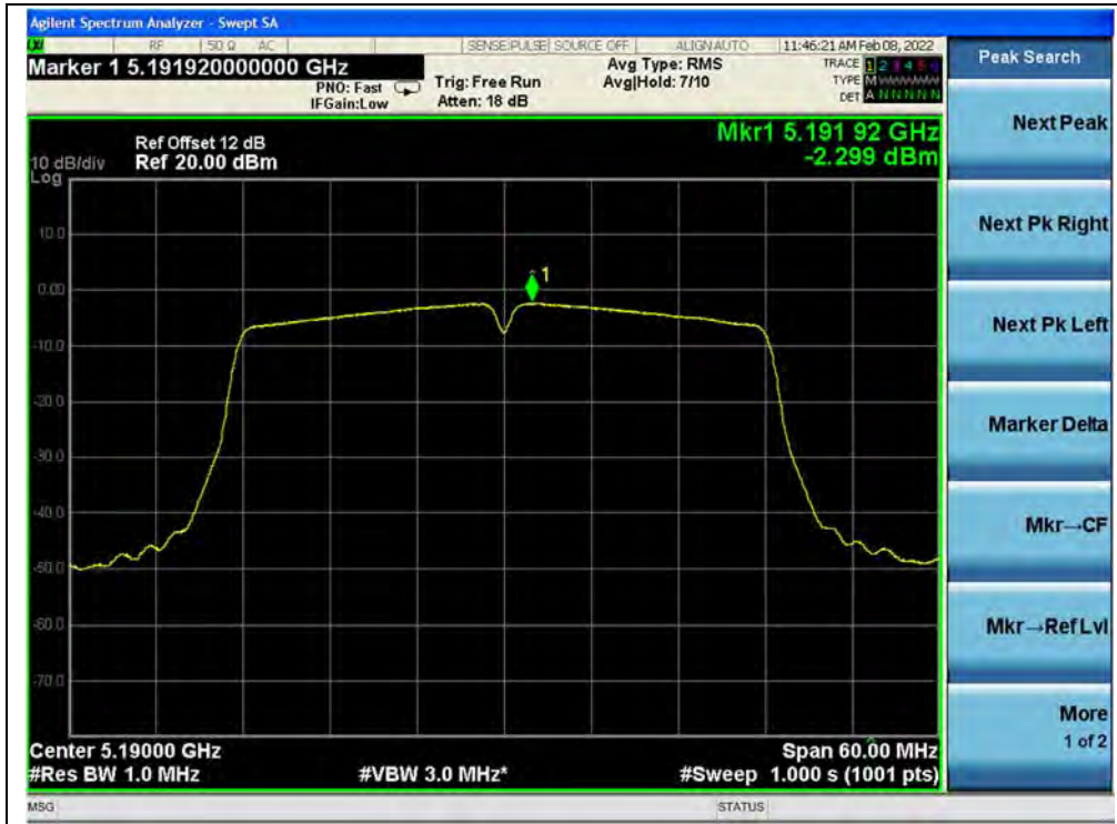
(Channel 38, 5190MHz, 802.11ac (VHT40))
