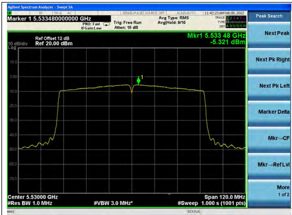
(Channel 106, 5530MHz, 802.11ac (VHT80))
