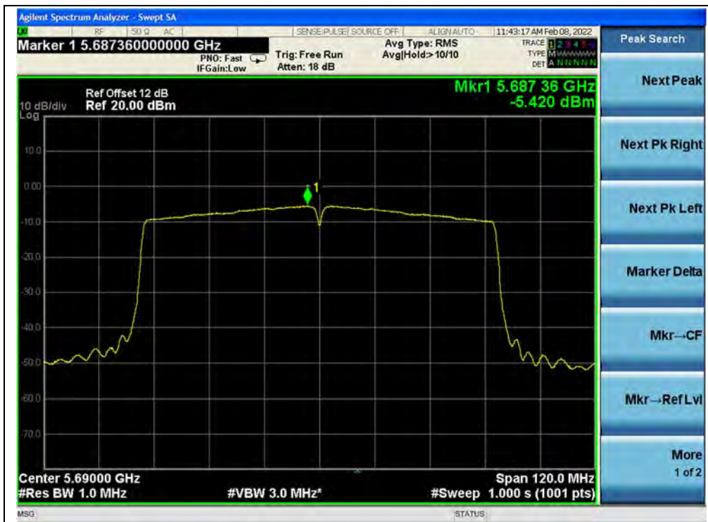
(Channel 138, 5690MHz, 802.11ac (VHT80))
