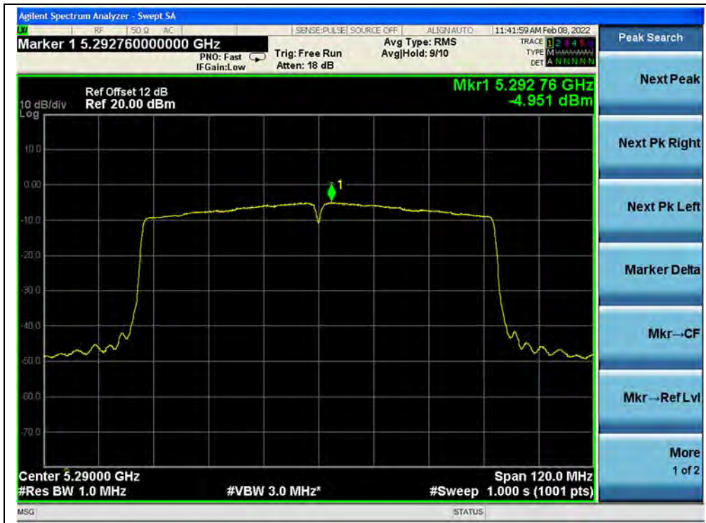
(Channel 58, 5290MHz, 802.11ac (VHT80))
