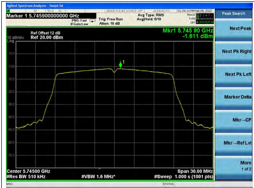
(Channel 149, 5745MHz, 802.11ac (VHT20))
