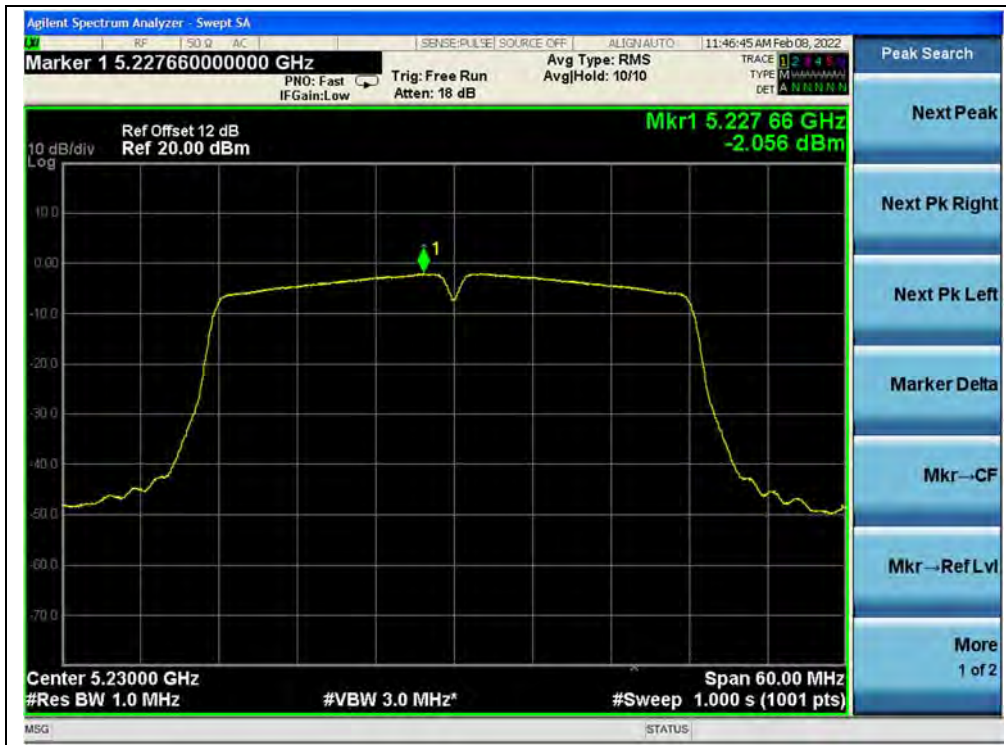
(Channel 46, 5230MHz, 802.11ac (VHT40))
