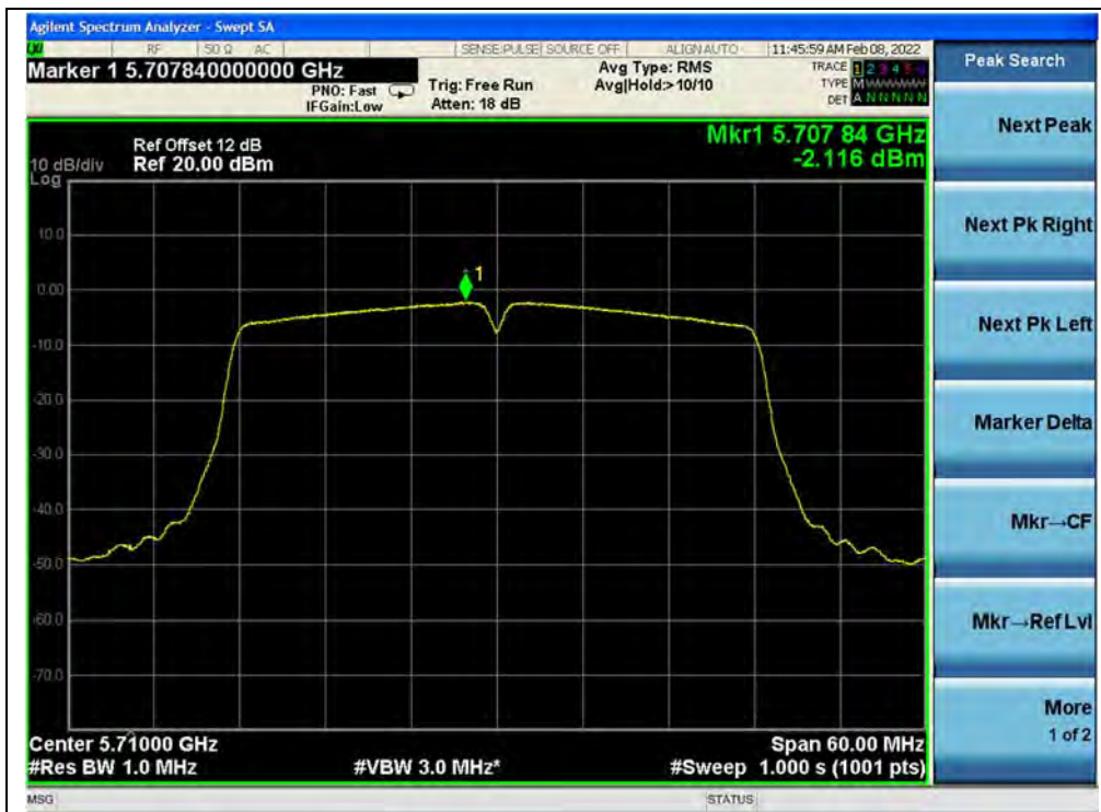
(Channel 142, 5710MHz, 802.11ac (VHT40))
