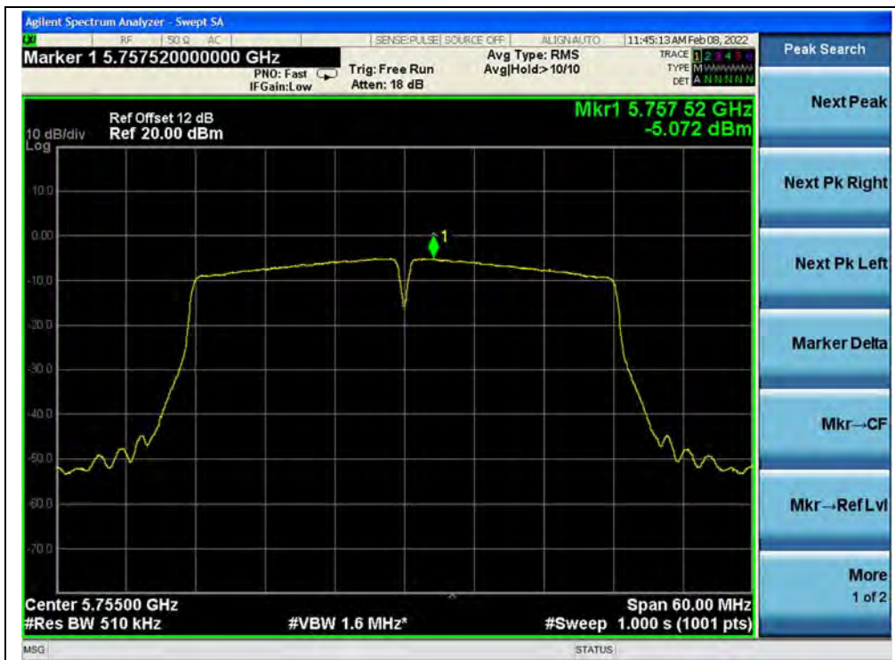
(Channel 151, 5755MHz, 802.11ac (VHT40))
