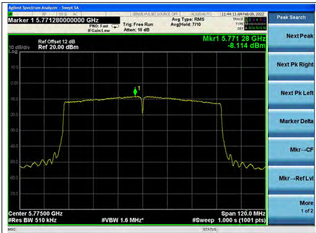
(Channel 155, 5775MHz, 802.11ac (VHT80))
