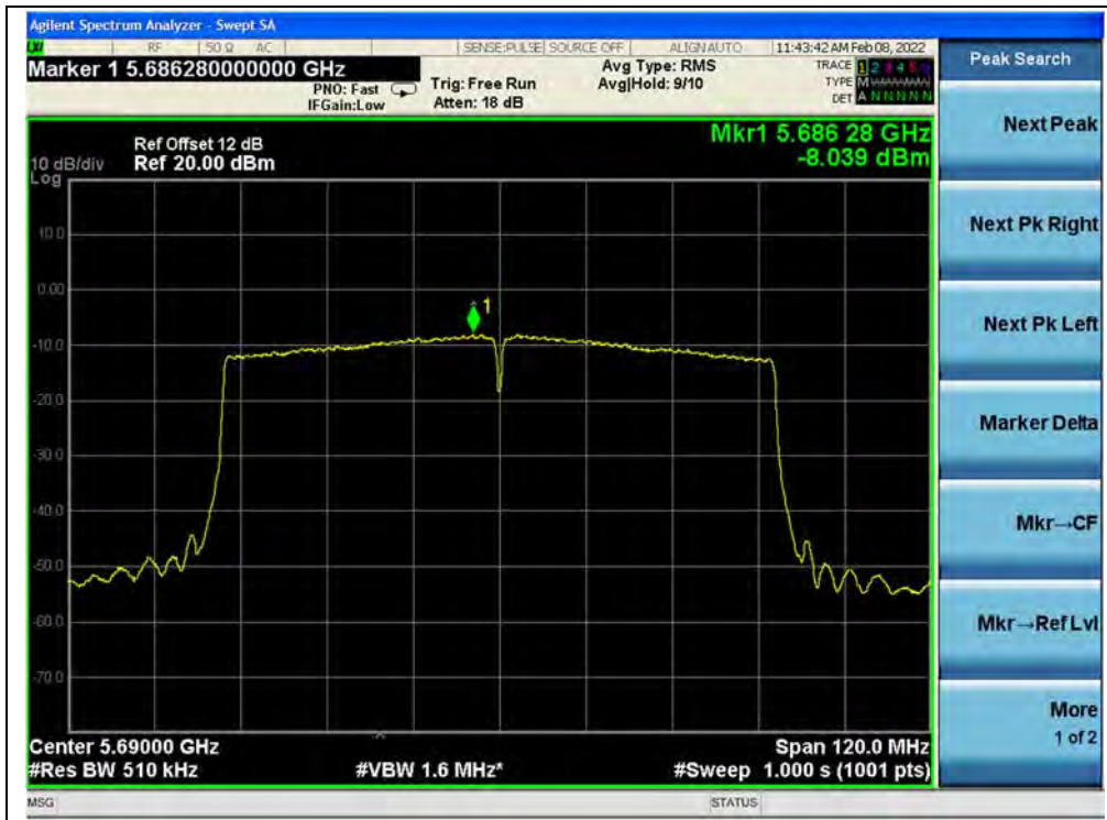
(Channel 138, 5690MHz, 802.11ac (VHT80))
