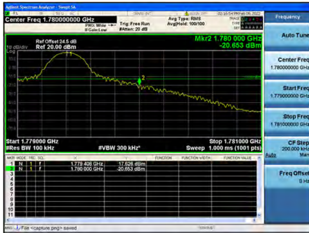
Band66 / 10MHz / High CH / QPSK / 1 RB
