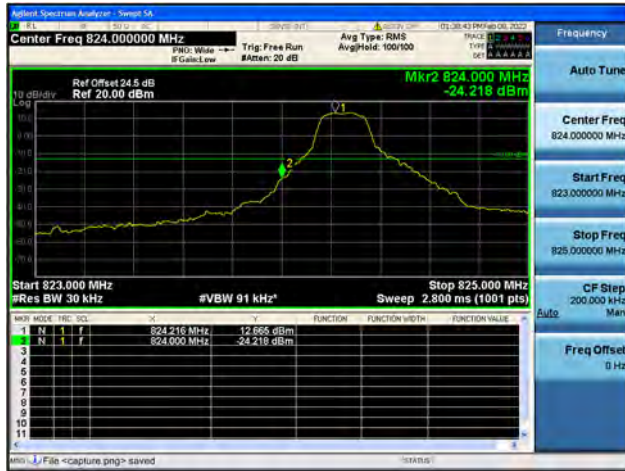
Band5 / 1.4MHz / High CH / QPSK / 1 RB
