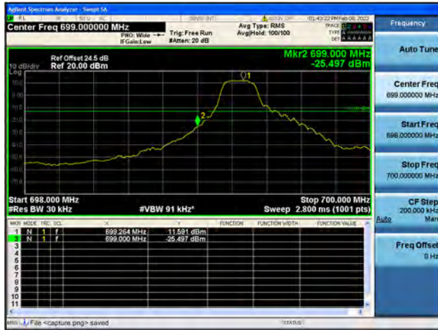
Band12 / 3MHz / High CH / QPSK / 1 RB
