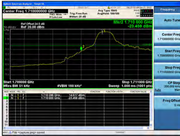
Band4 / 5MHz / High CH / QPSK / 1 RB
