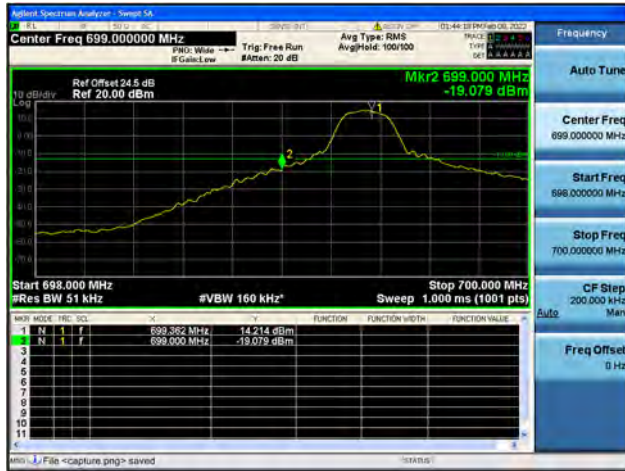
Band12 / 5MHz / High CH / QPSK / 1 RB
