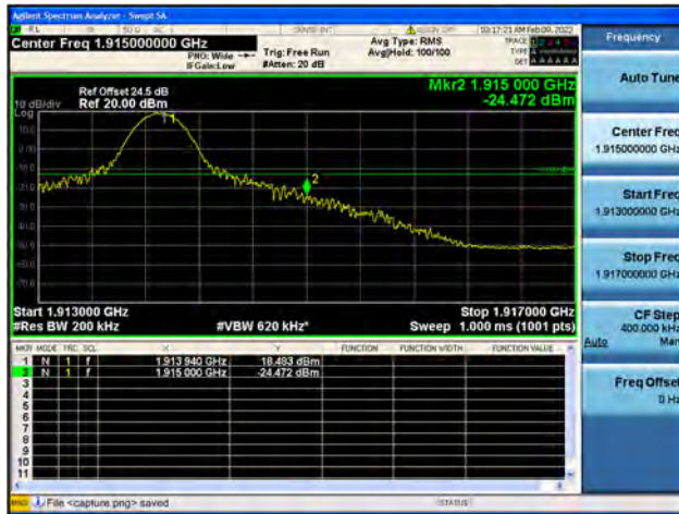
Band25 / 20MHz / High CH / QPSK / 1 RB
