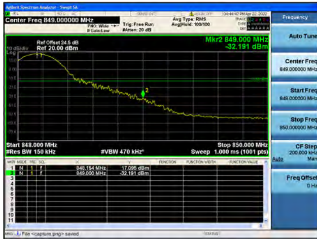
Band26 / 15MHz / High CH / QPSK / 1 RB
