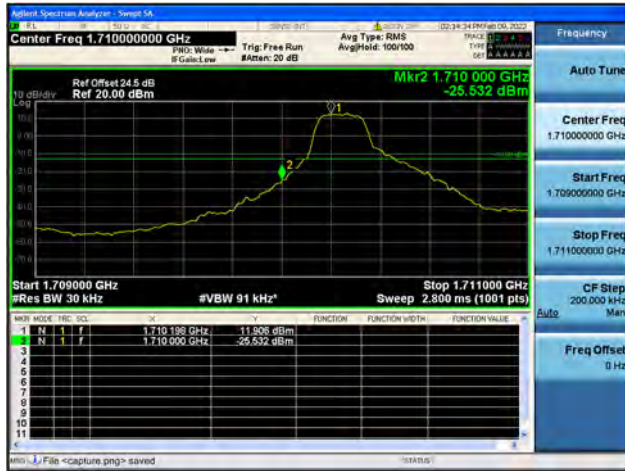
Band66 / 3MHz / High CH / QPSK / 1 RB
