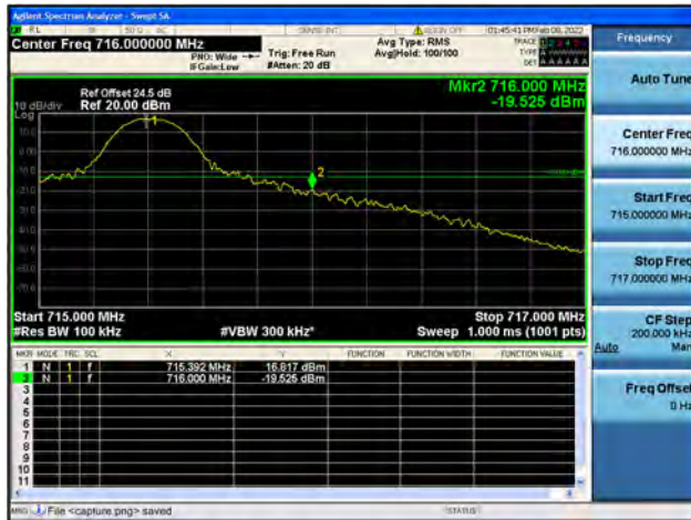
Band12 / 10MHz / High CH / QPSK / 1 RB
