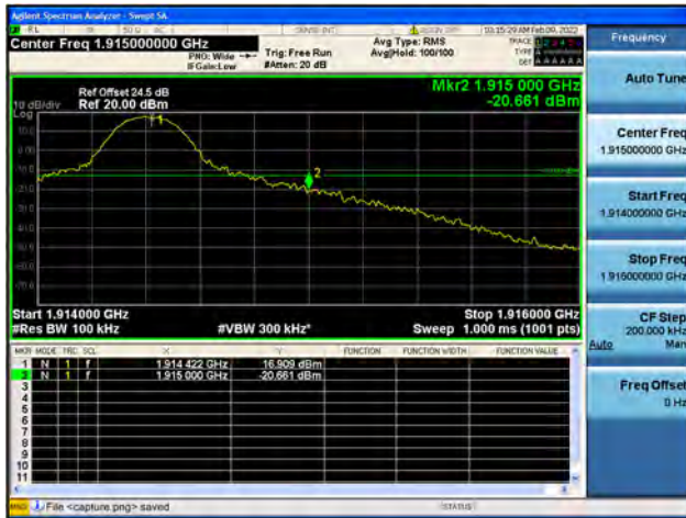
Band25 / 10MHz / High CH / QPSK / 1 RB
