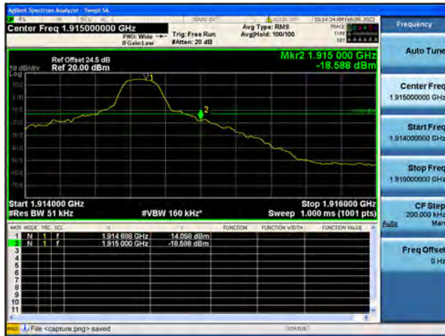
Band25 / 5MHz / High CH / QPSK / 1 RB
