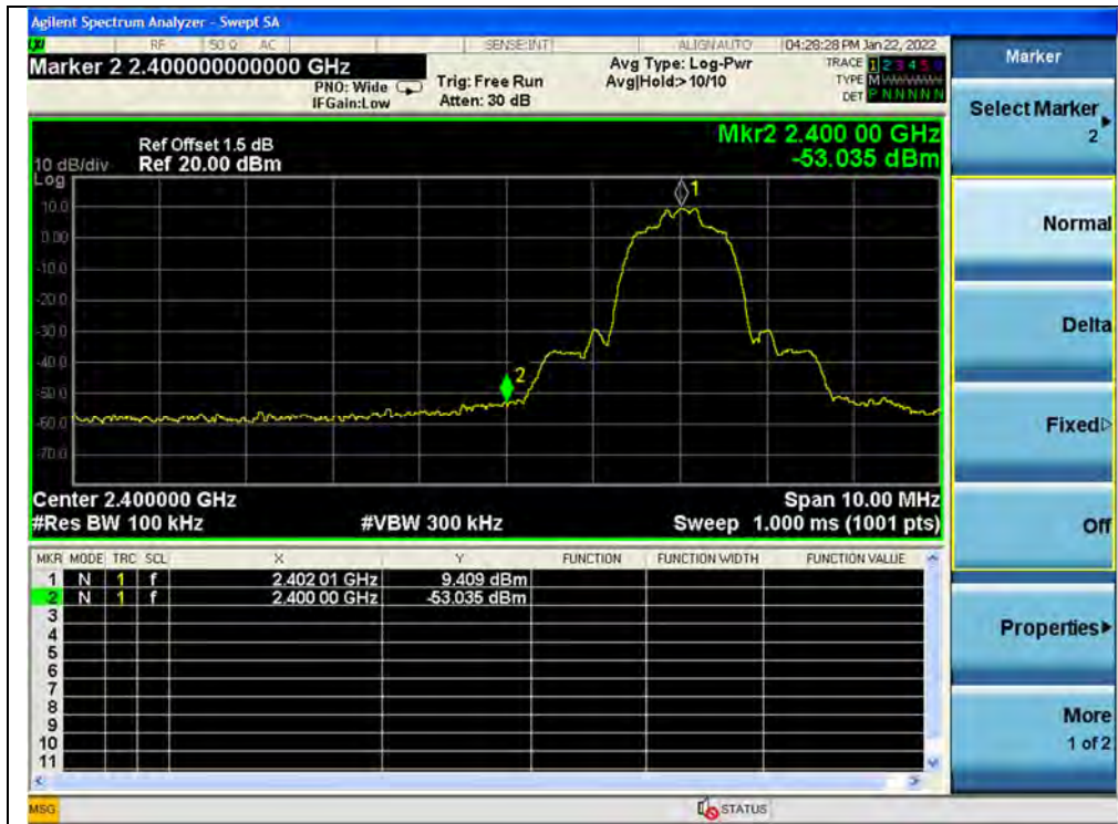
(Band edge, Channel 0, \pi/4 -DQPSK)
