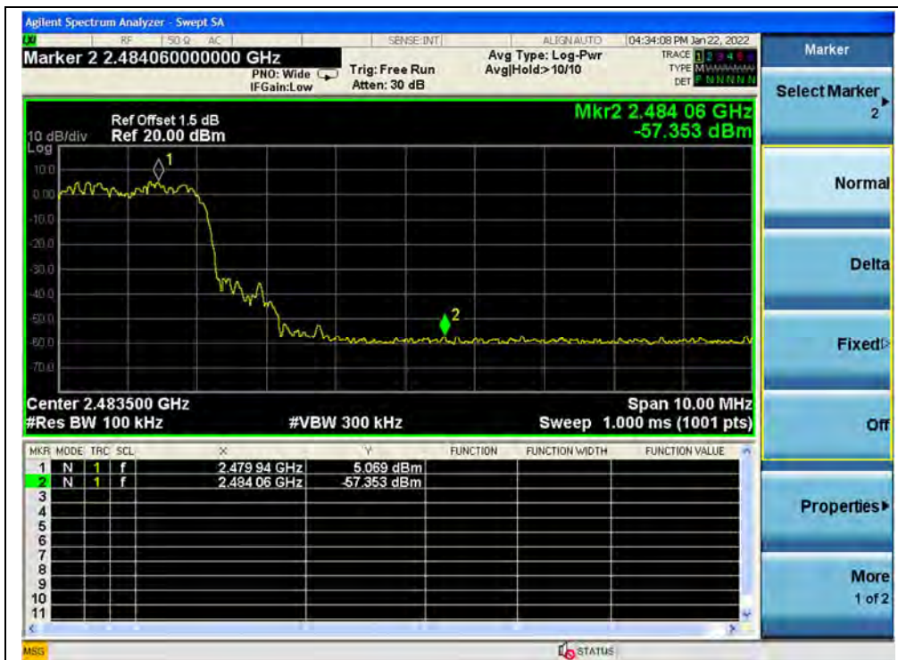
(Band edge with hopping on, Channel 78, 8-DPSK)
