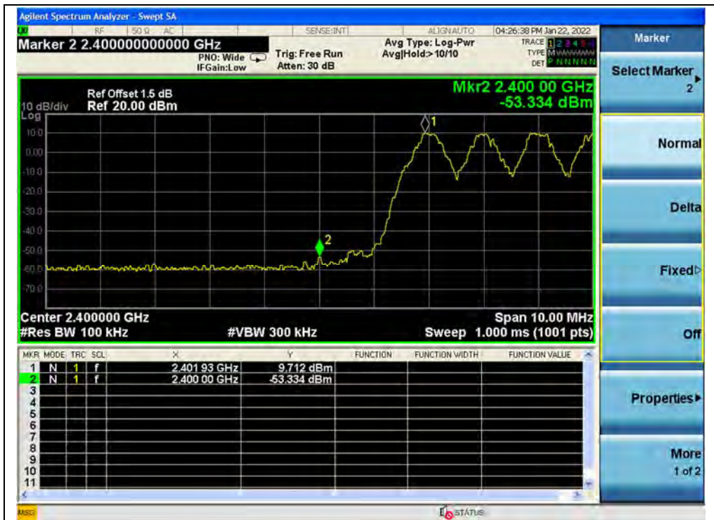
(Band edge with hopping on, Channel 0, GFSK)
