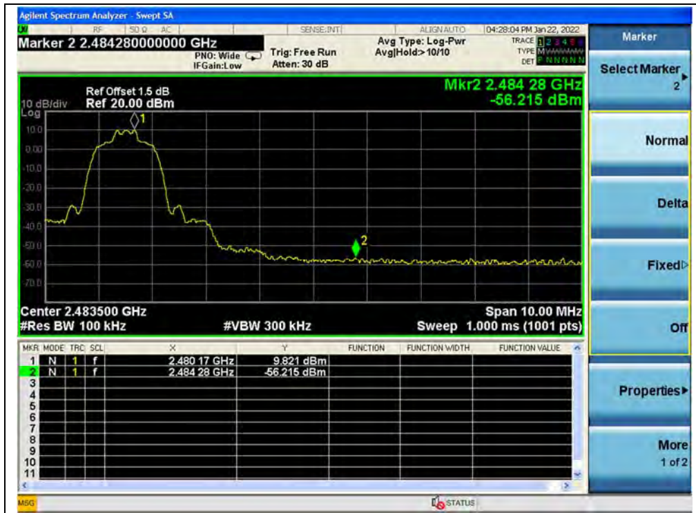
(Band edge, Channel 78, \pi/4 -DQPSK)
