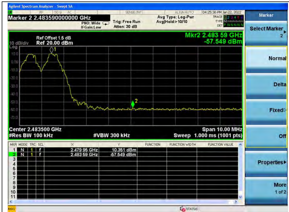
(Band edge with hopping on, Channel 78, GFSK)
