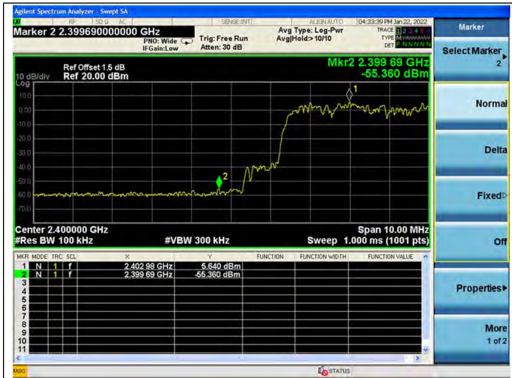
(Band edge with hopping on, Channel 0, 8-DPSK)
