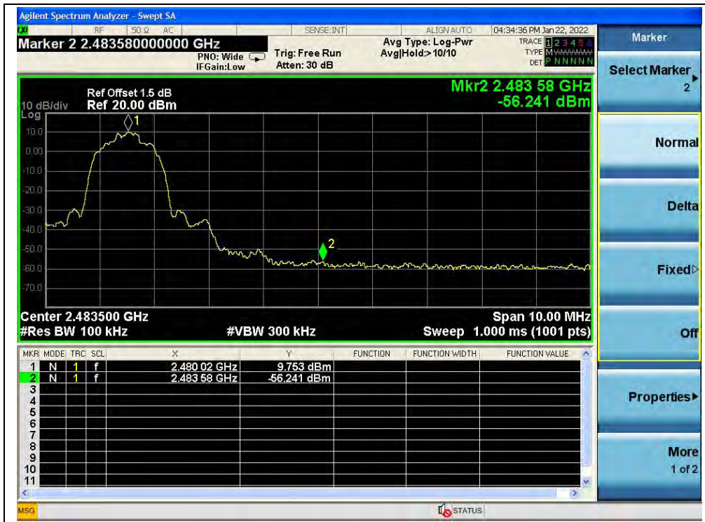
(Band edge, Channel 78, 8-DPSK)
