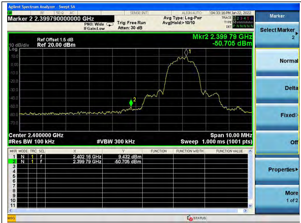
(Band edge, Channel 0, 8-DPSK)
