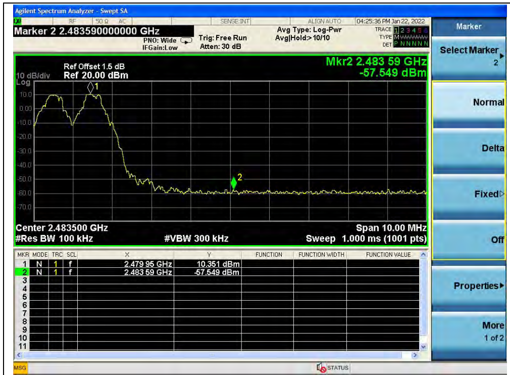
(Band edge with hopping on, Channel 78, GFSK)
