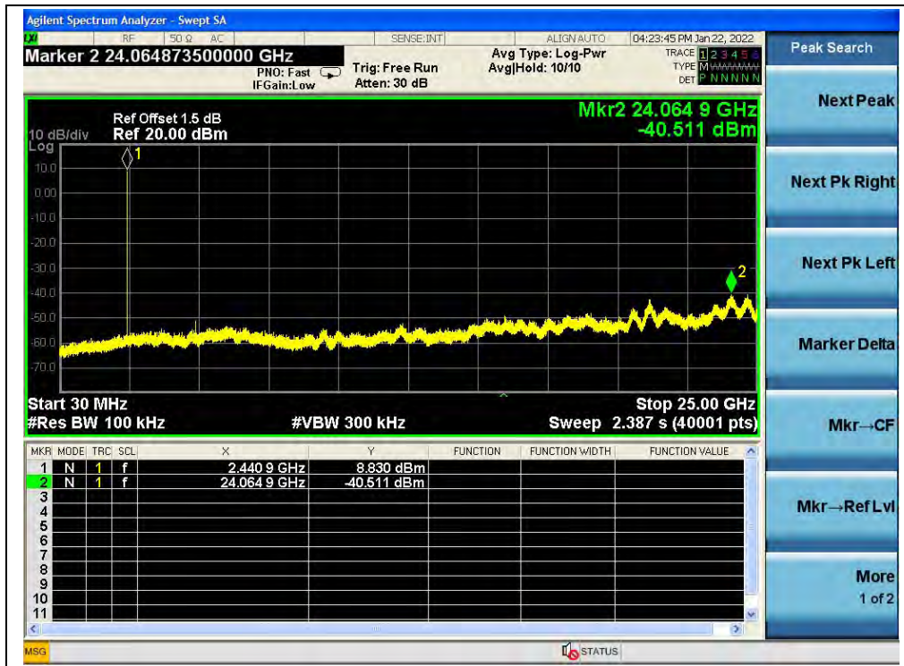
(30MHz to 25GHz, Channel 39, GFSK)
