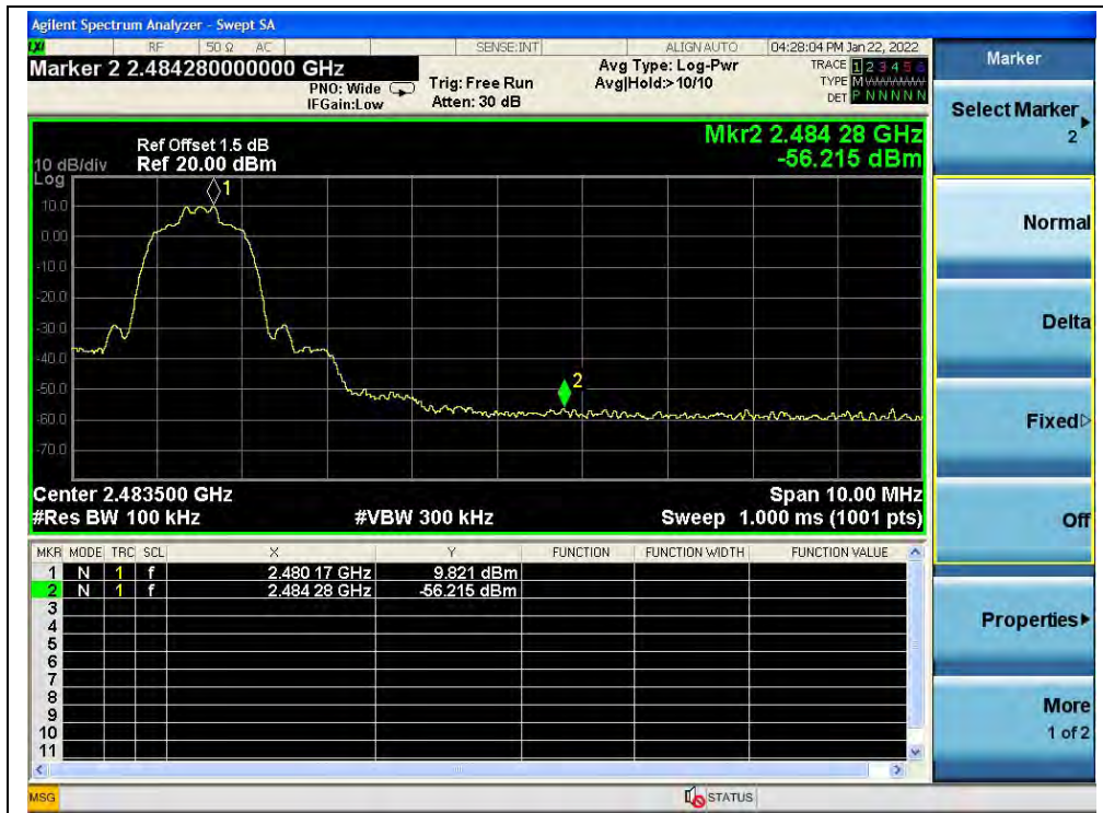
(Band edge, Channel 78, \pi/4 -DQPSK)
