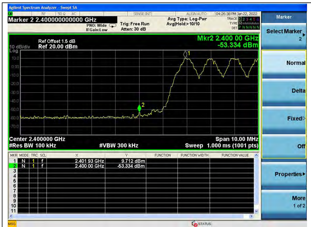
(Band edge with hopping on, Channel 0, GFSK)
