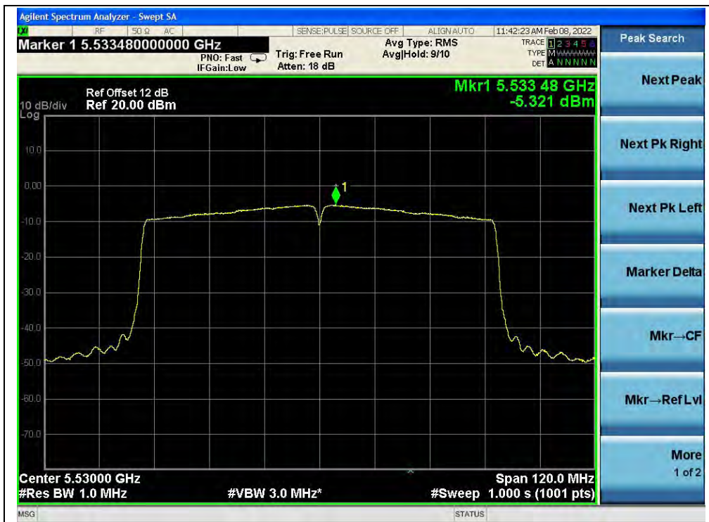
(Channel 106, 5530MHz, 802.11ac (VHT80))
