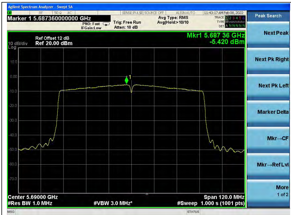
(Channel 138, 5690MHz, 802.11ac (VHT80))
