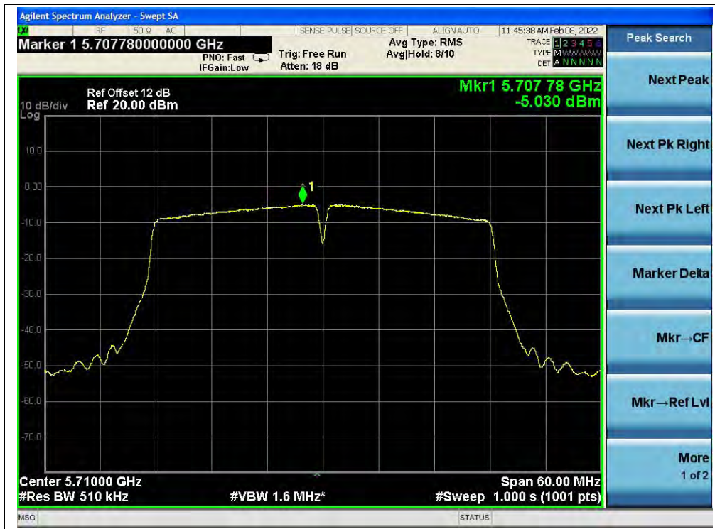
(Channel 142, 5710MHz, 802.11ac (VHT40))
