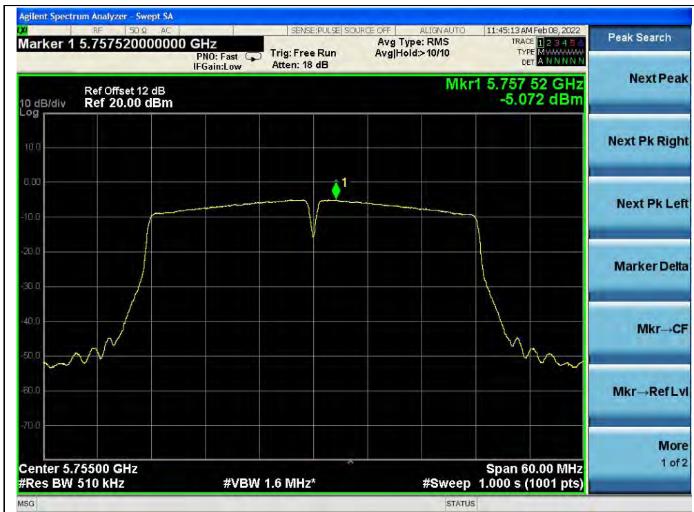
(Channel 151, 5755MHz, 802.11ac (VHT40))
