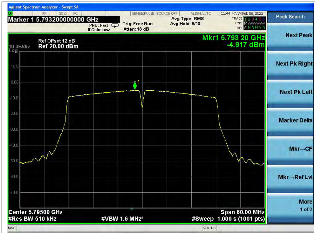
(Channel 159, 5795MHz, 802.11ac (VHT40))
