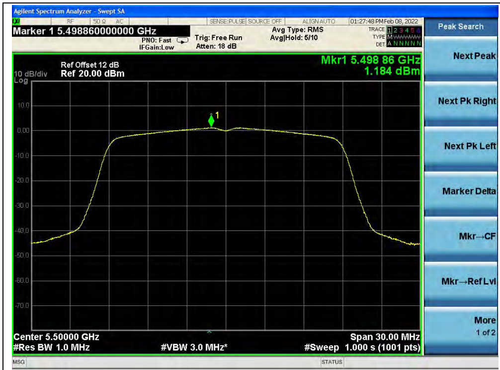
(Channel 100, 5500MHz, 802.11ac (VHT20))
