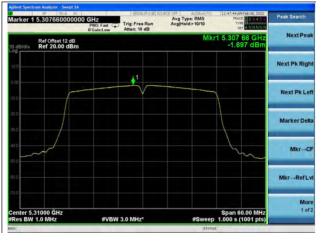
(Channel 62, 5310MHz, 802.11ac (VHT40))
