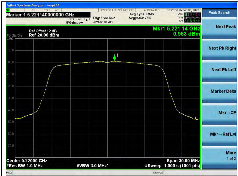
(Channel 44, 5220MHz, 802.11ac (VHT20))
