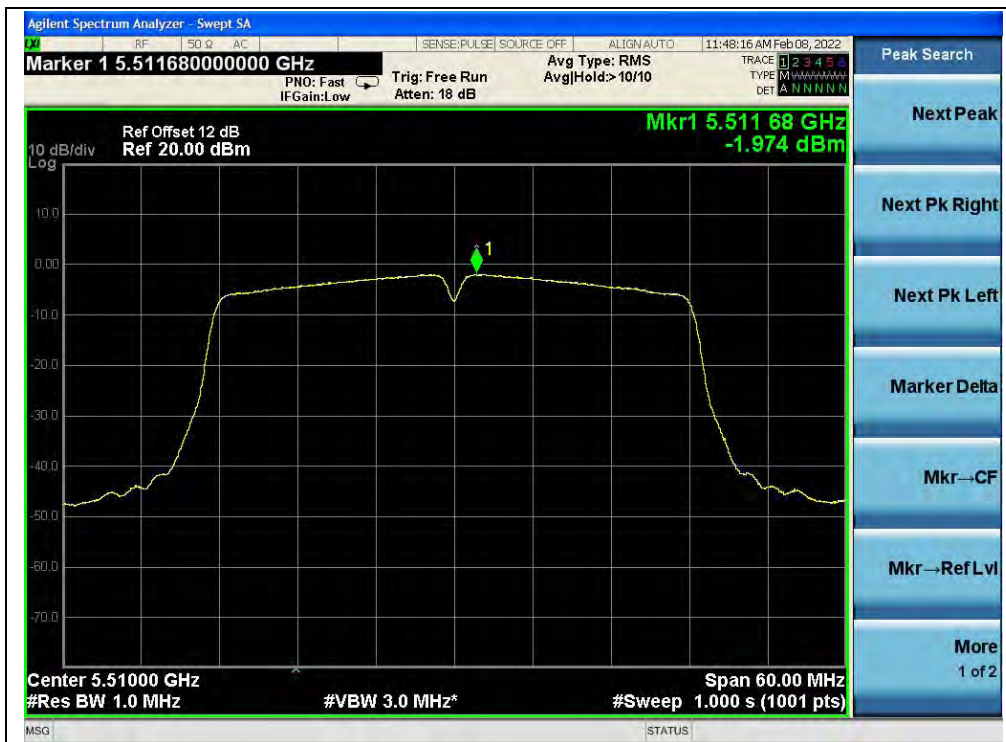
(Channel 102, 5510MHz, 802.11ac (VHT40))
