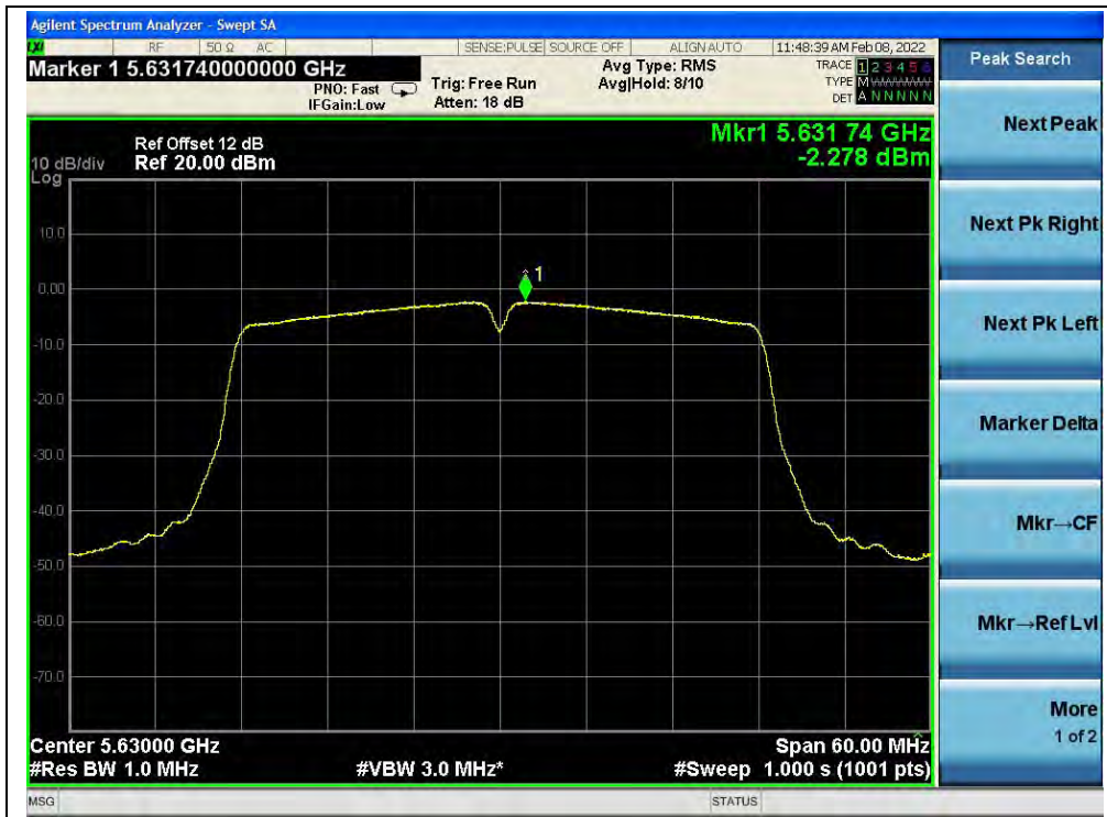
(Channel 126, 5630MHz, 802.11ac (VHT40))
