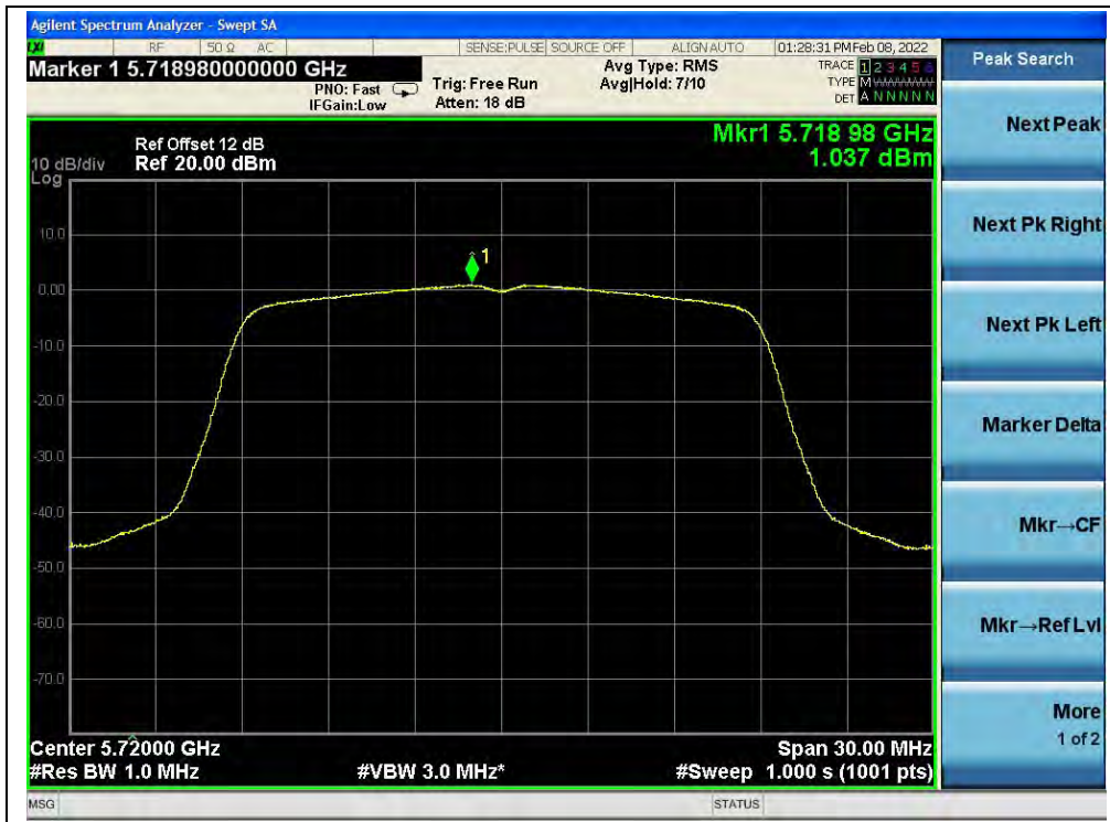
(Channel 144, 5720MHz, 802.11ac (VHT20))
