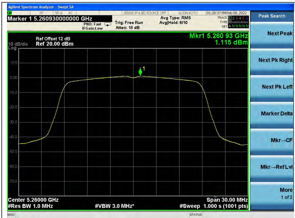
(Channel 52, 5260MHz, 802.11ac (VHT20))
