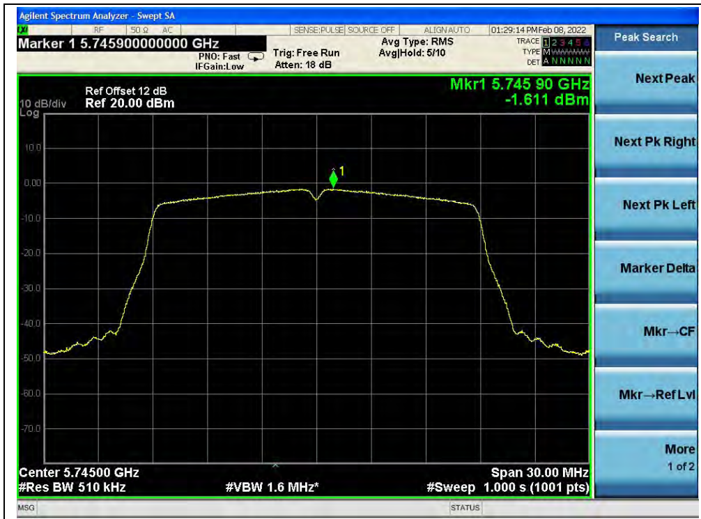
(Channel 149, 5745MHz, 802.11ac (VHT20))
