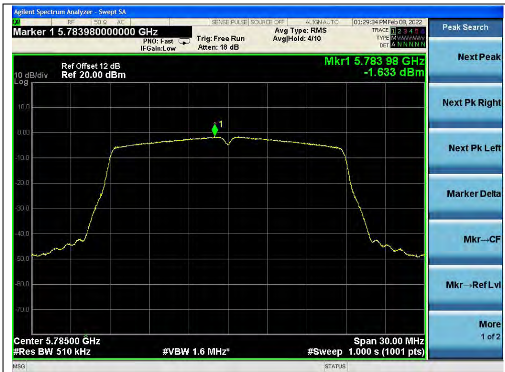
(Channel 157, 5785MHz, 802.11ac (VHT20))
