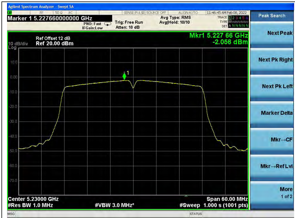
(Channel 46, 5230MHz, 802.11ac (VHT40))
