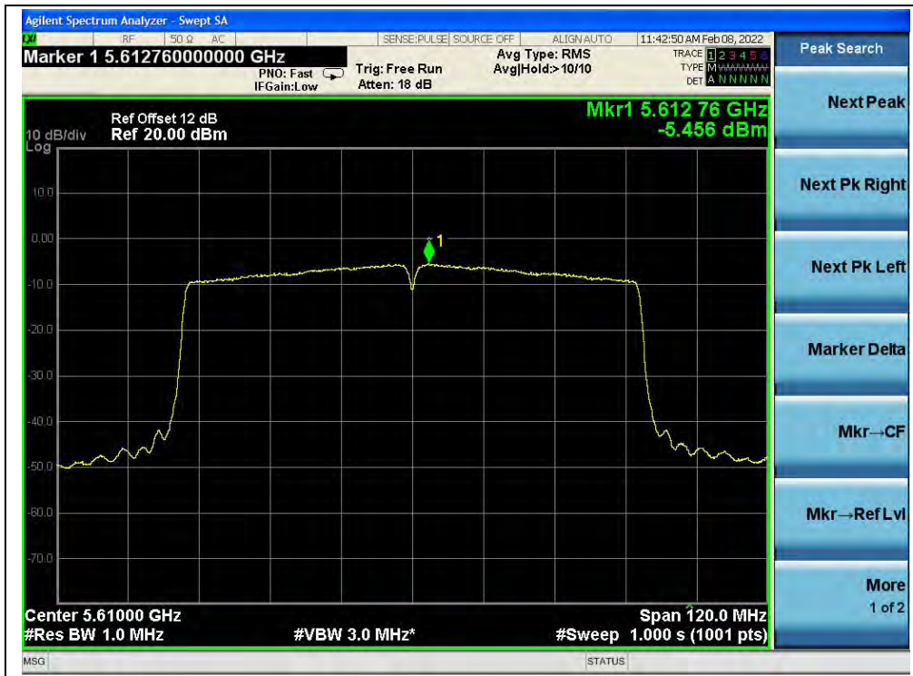
(Channel 122, 5610MHz, 802.11ac (VHT80))
