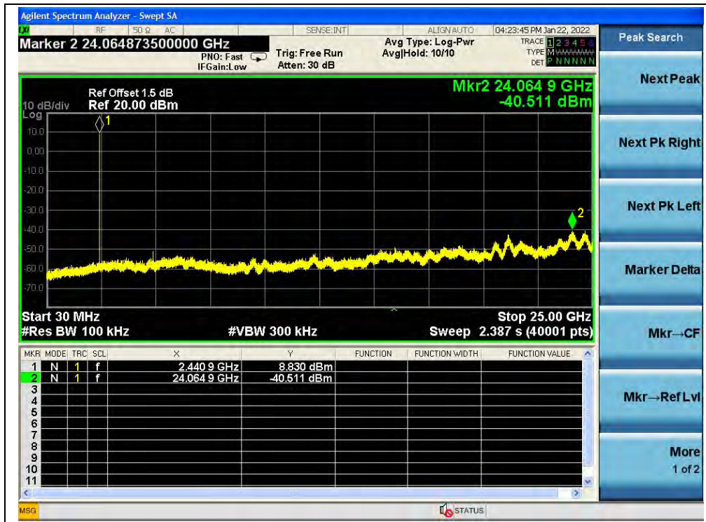
(30MHz to 25GHz, Channel 39, GFSK)
