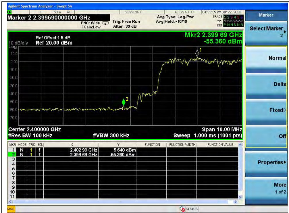
(Band edge with hopping on, Channel 0, 8-DPSK)
