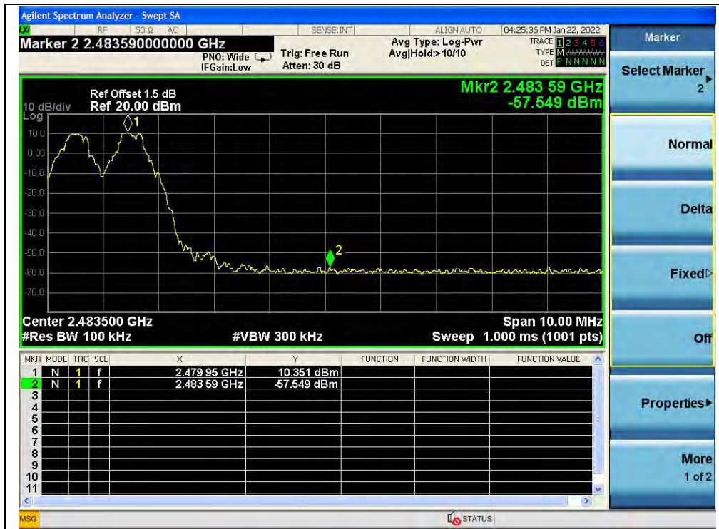
(Band edge with hopping on, Channel 78, GFSK)
