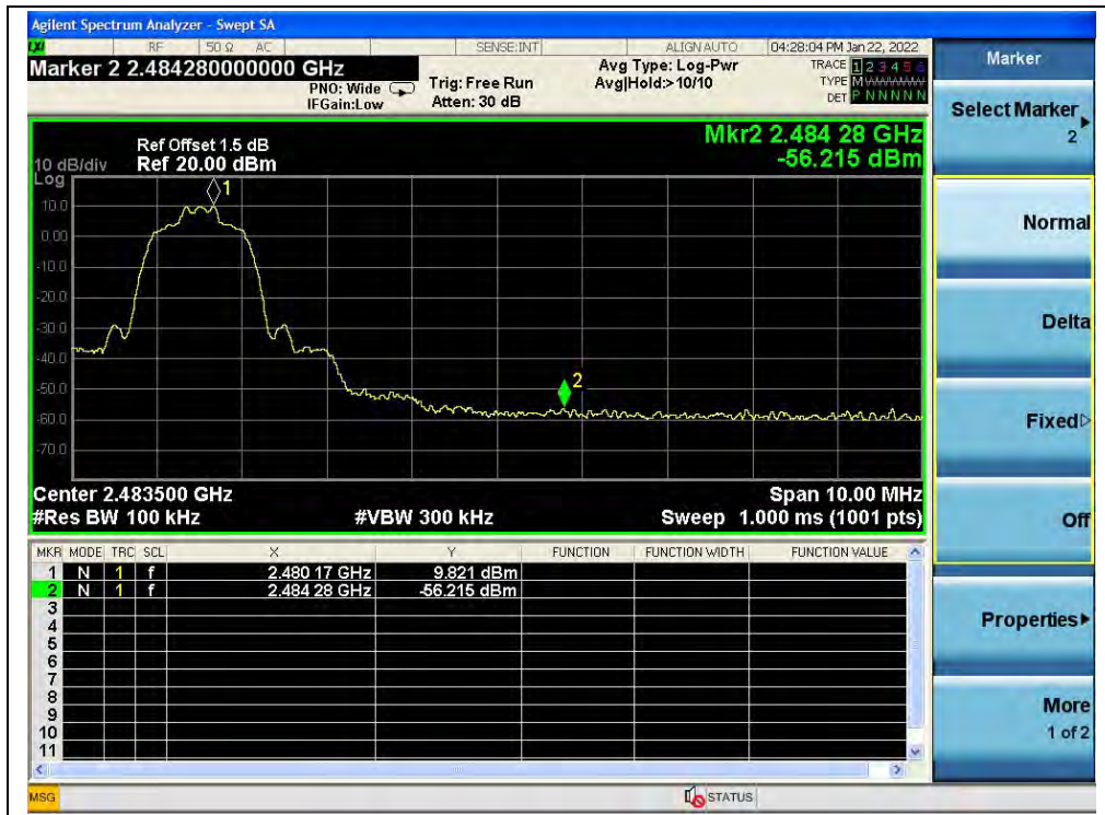
(Band edge, Channel 78, \pi/4 -DQPSK)
