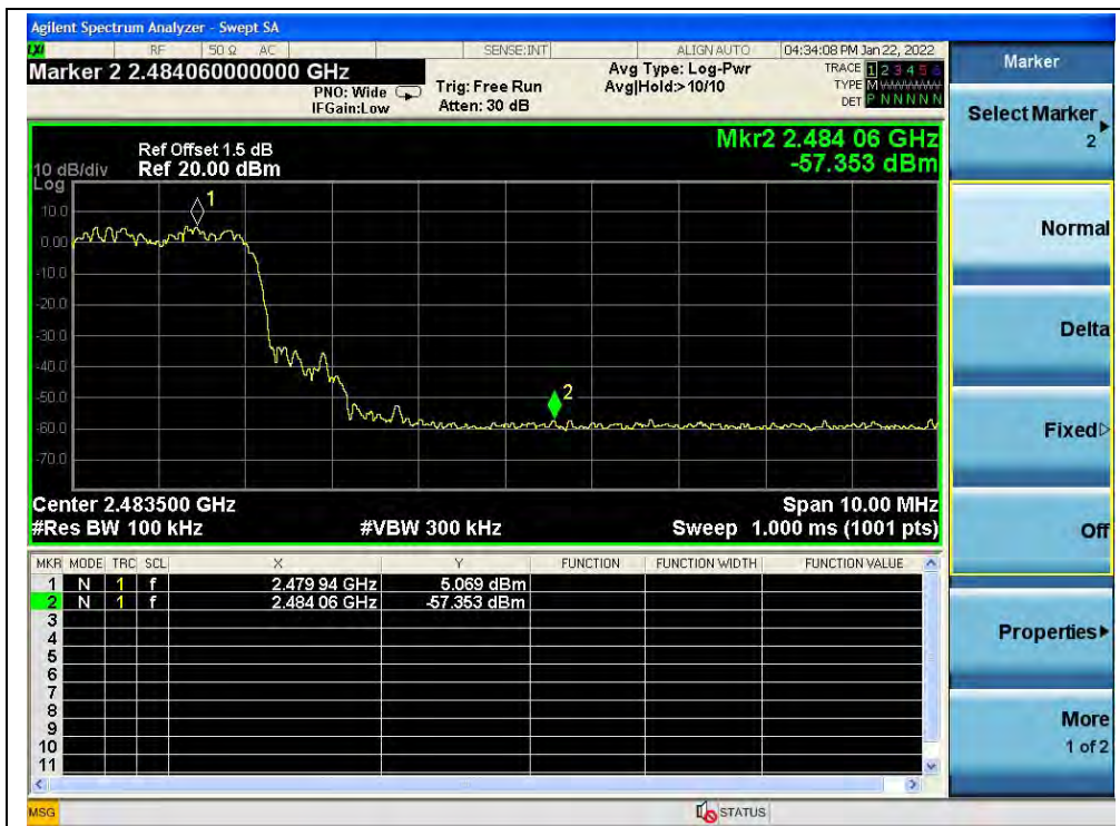
(Band edge with hopping on, Channel 78, 8-DPSK)
