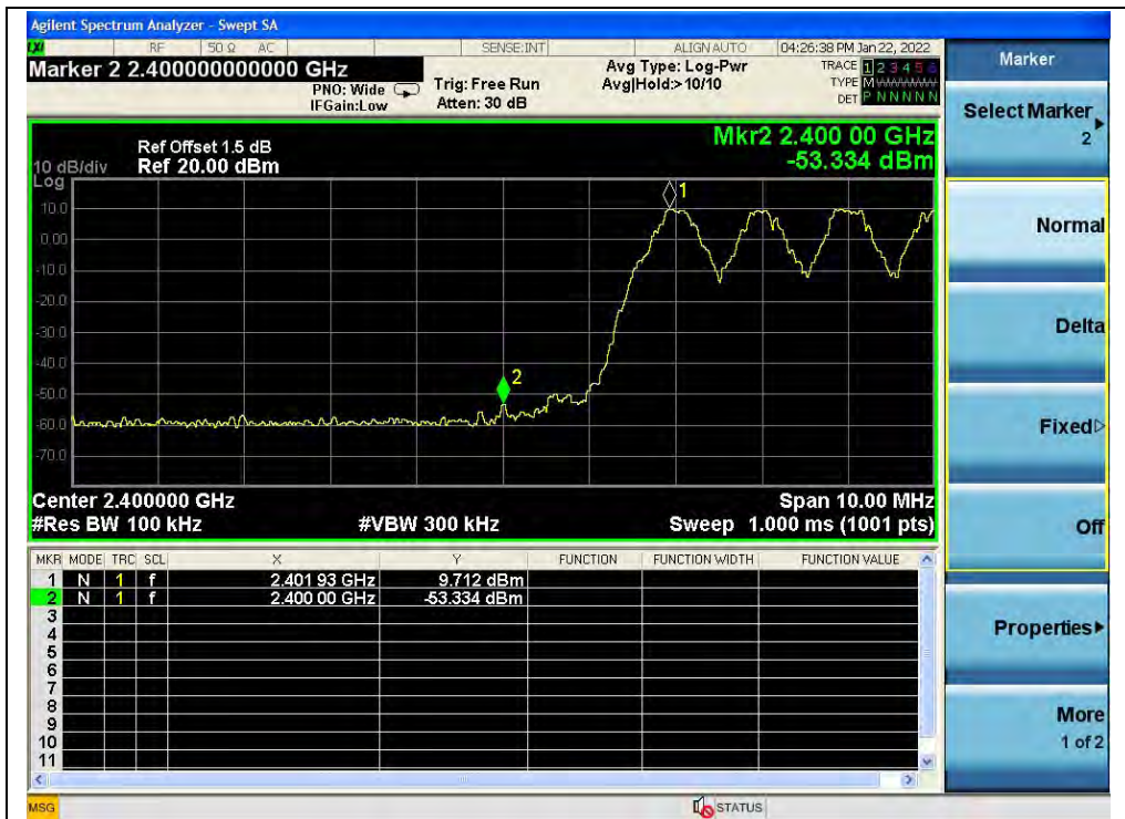
(Band edge with hopping on, Channel 0, GFSK)
