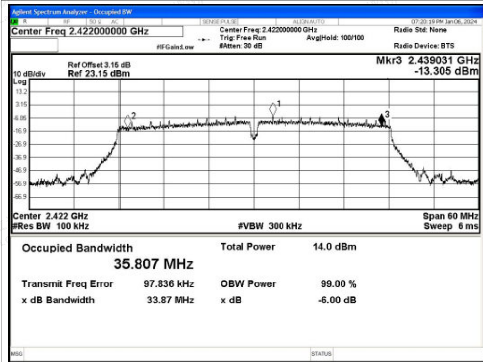
-6dB Bandwidth NVNT n40 2422MHz Ant1
