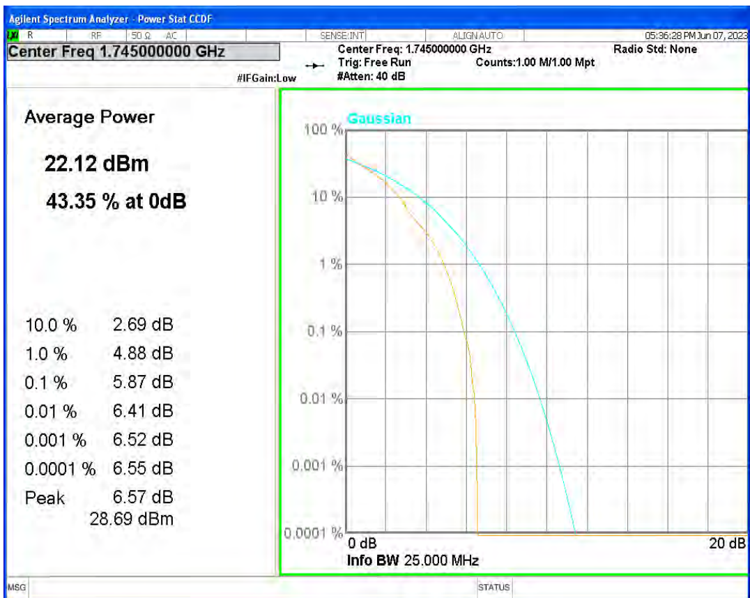
Band66 QPSK BW=20MHz Channel=132572 RB Size=1 Position=#0
