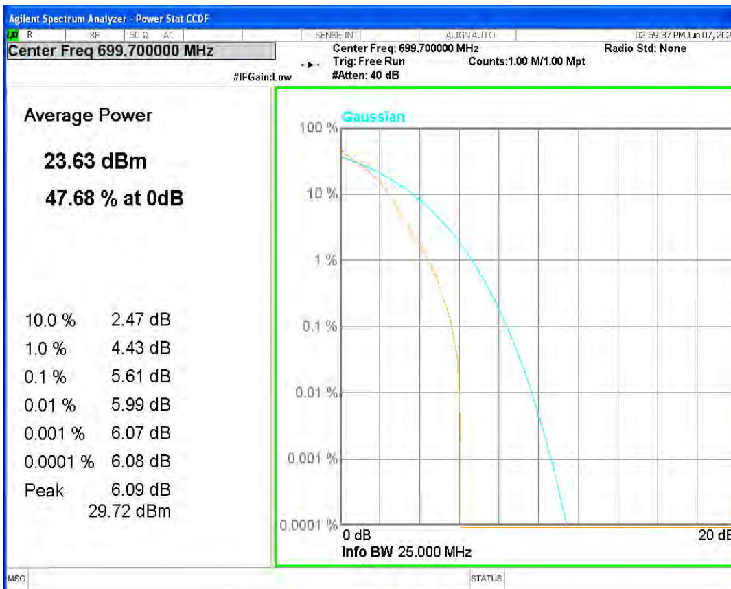
Band12 QPSK BW=1.4MHz Channel=23095 RB Size=1 Position=#0
