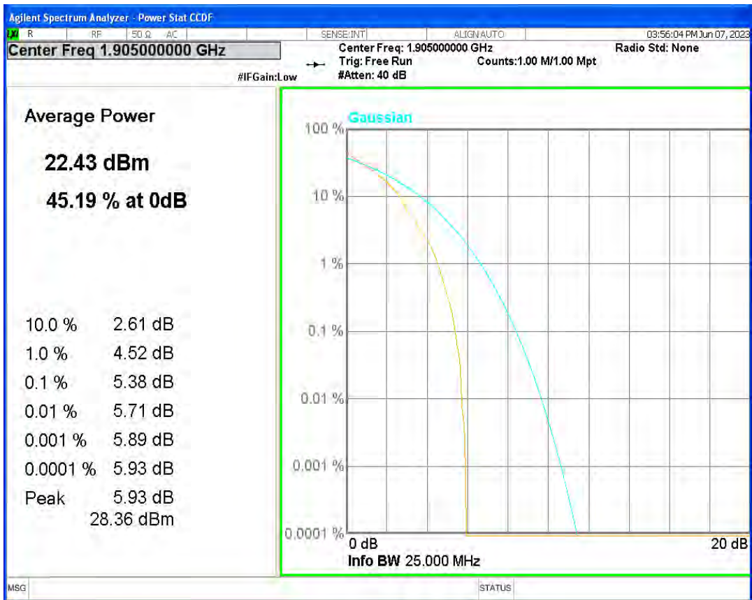
Band25 QPSK BW=3MHz Channel=26055 RB Size=1 Position=#0
