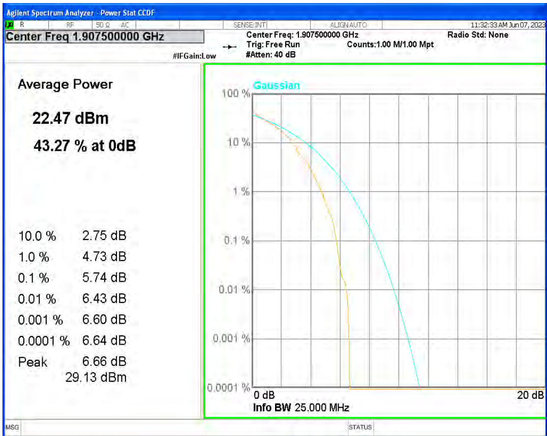
Band25 16QAM BW=1.4MHz Channel=26047 RB Size=1 Position=#0
