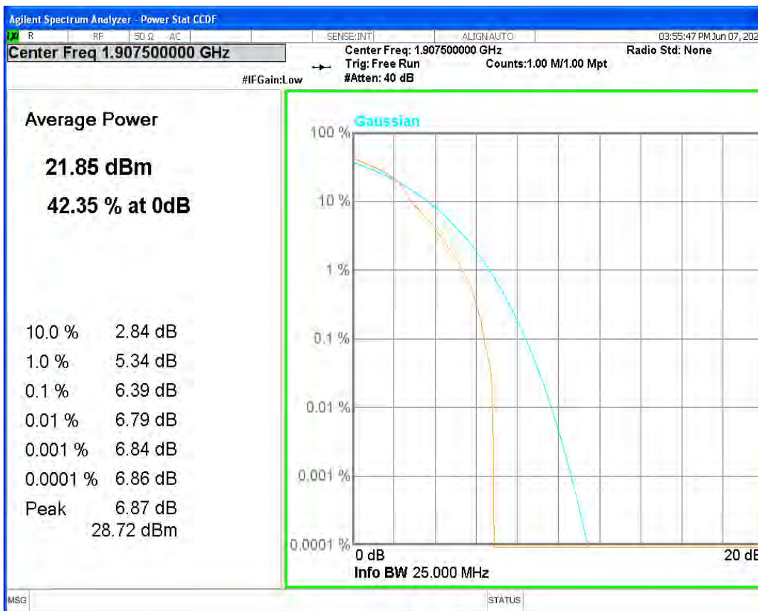
Band25 16QAM BW=20MHz Channel=26140 RB Size=1 Position=#0
