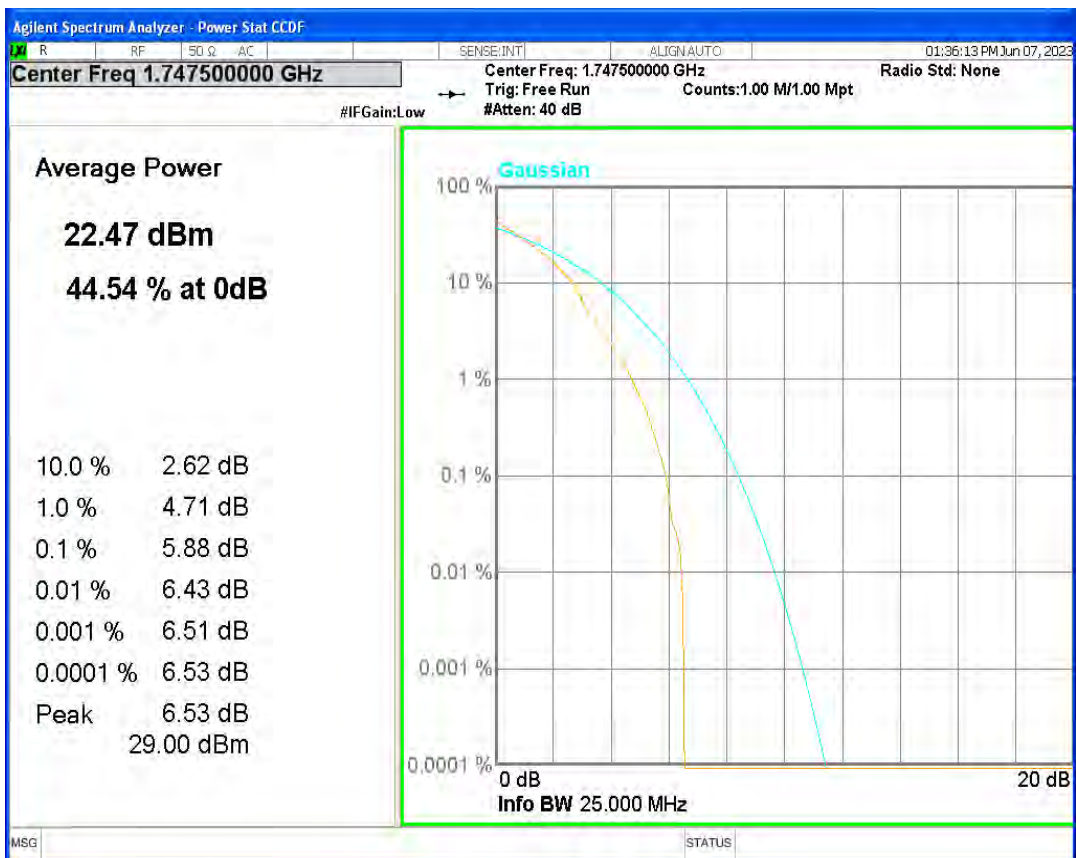
Band4 QPSK BW=20MHz Channel=20050 RB Size=1 Position=#0
