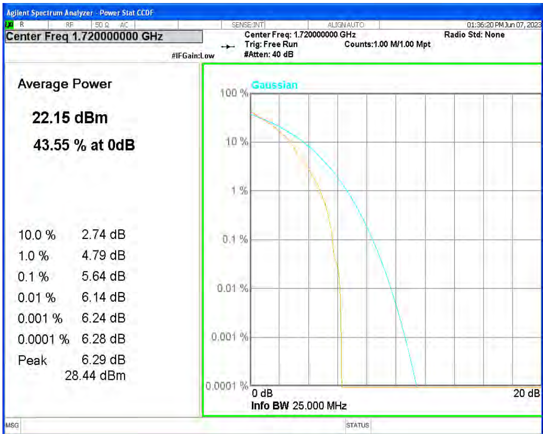
Band4 QPSK BW=20MHz Channel=20175 RB Size=1 Position=#0
