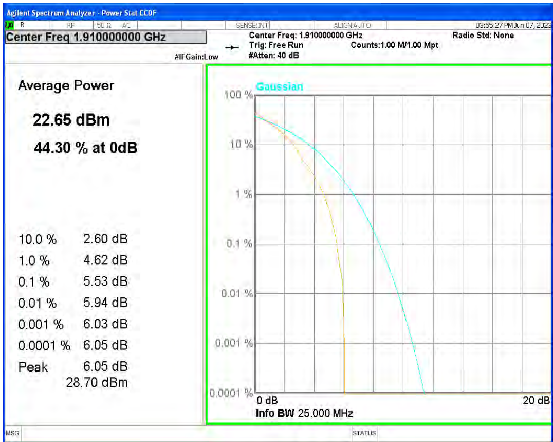
Band25 QPSK BW=15MHz Channel=26115 RB Size=1 Position=#0
