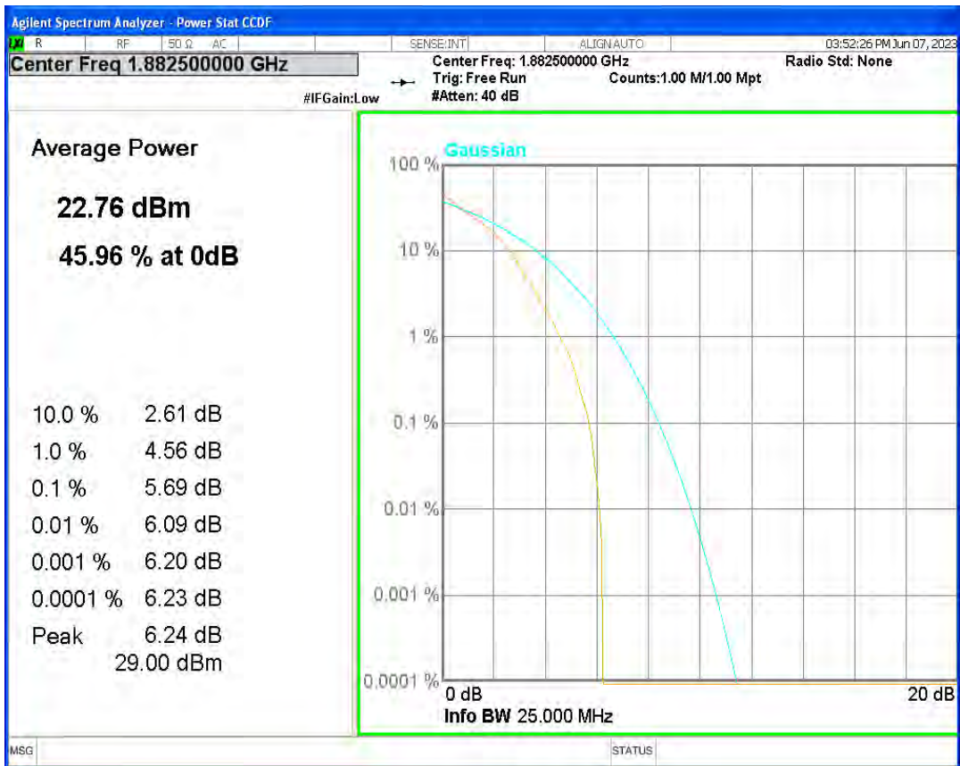
Band25 QPSK BW=1.4MHz Channel=26683 RB Size=1 Position=#0
