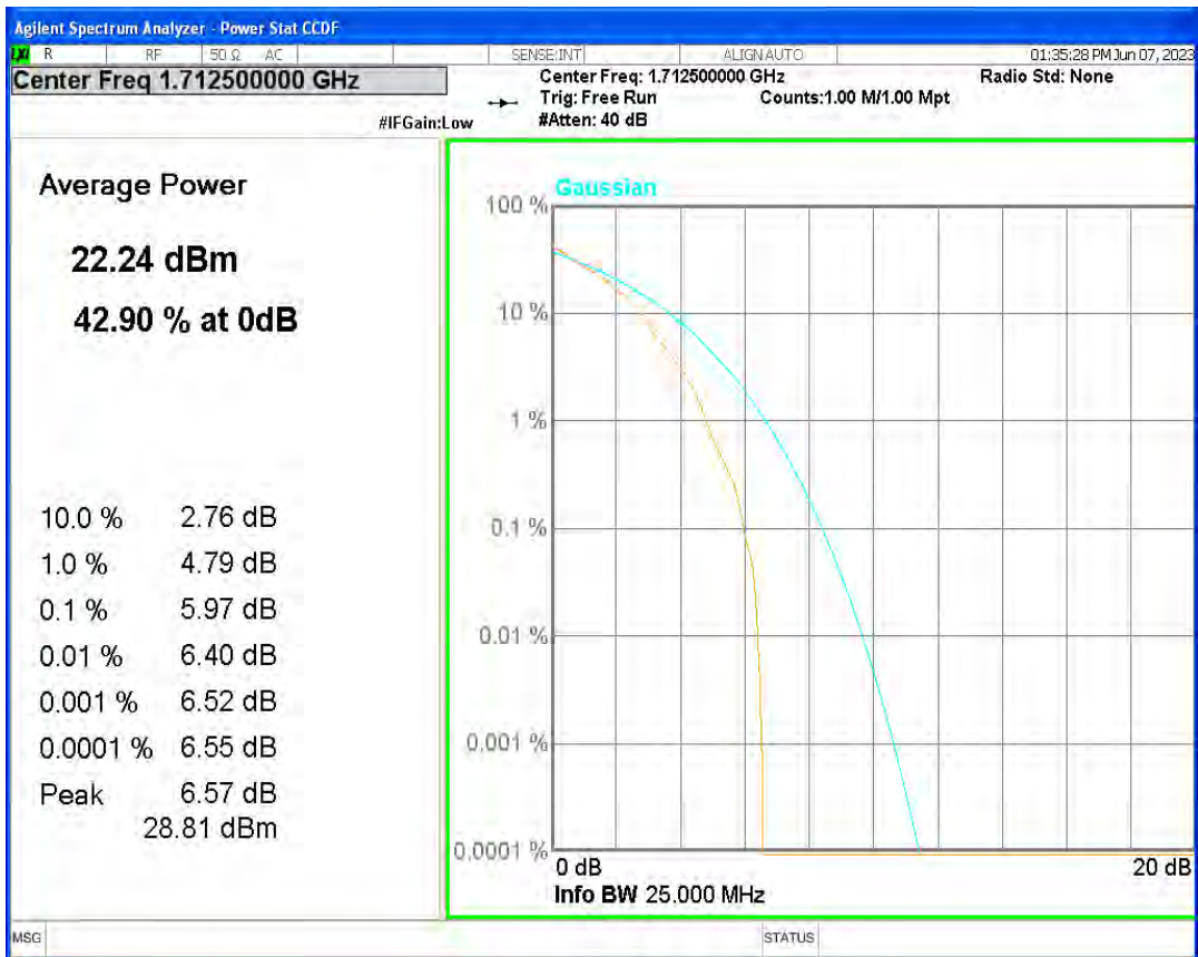
Band4 QPSK BW=5MHz Channel=20175 RB Size=1 Position=#0
