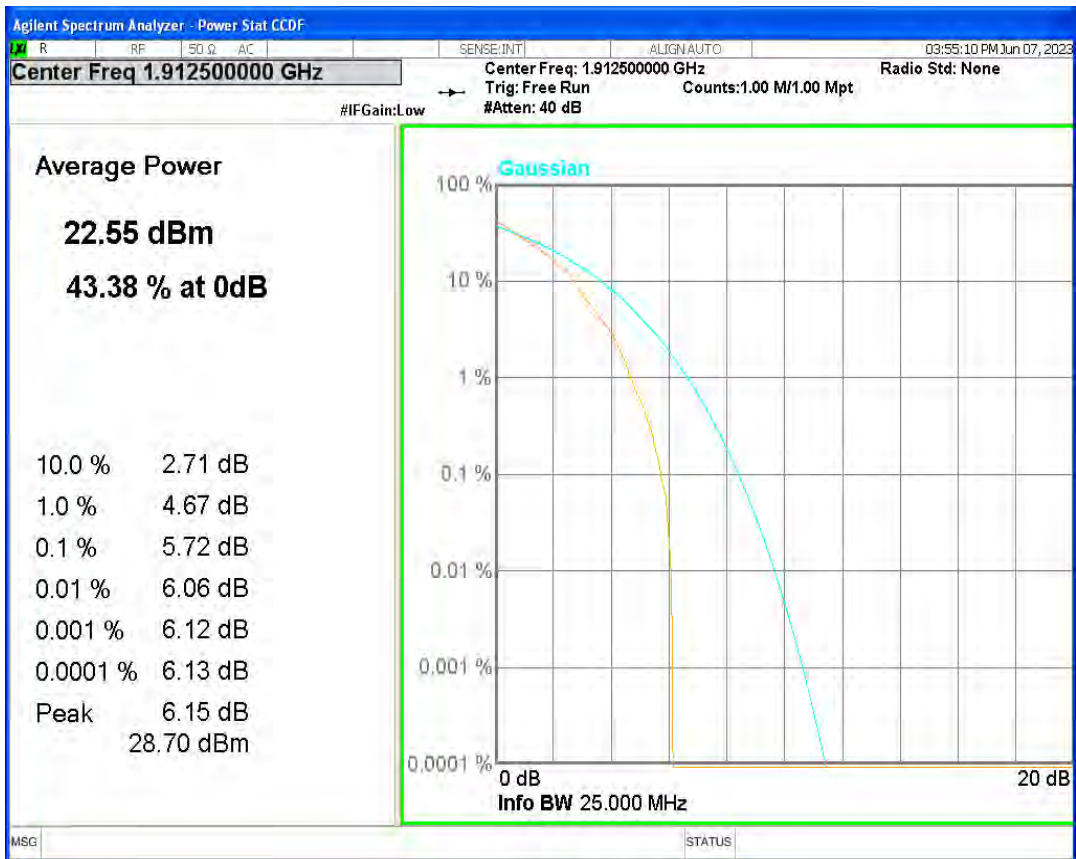
Band26(814-824) 16QAM BW=1.4MHz Channel=26697 RB Size=1 Position=#0
