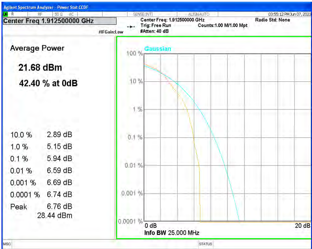
Band25 QPSK BW=1.4MHz Channel=26047 RB Size=1 Position=#0
