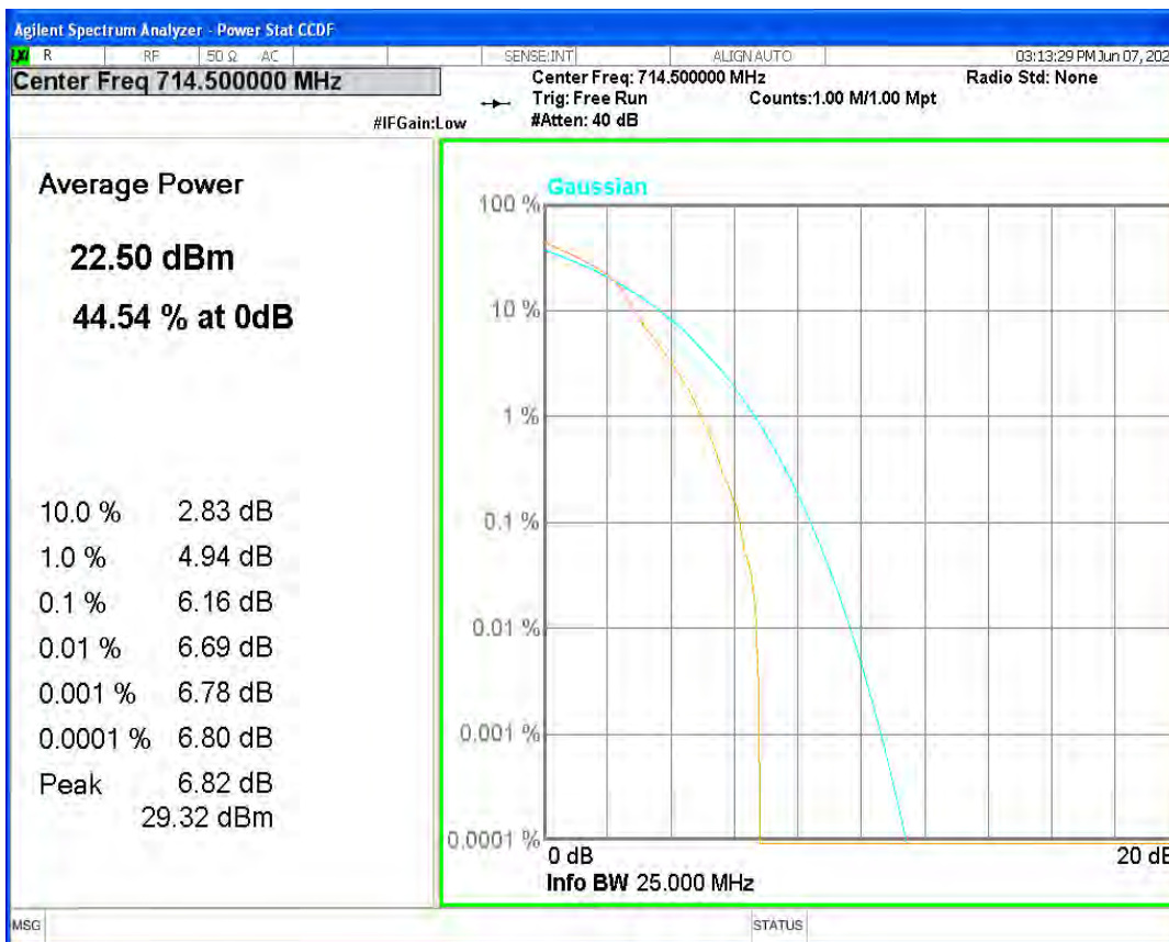
Band12 16QAM BW=5MHz Channel=23035 RB Size=1 Position=#0
