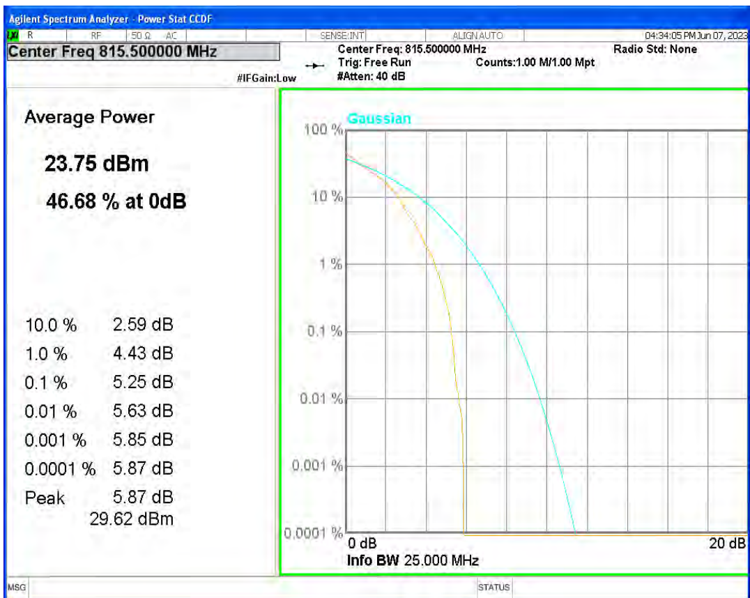
Band26(814-824) QPSK BW=3MHz Channel=26740 RB Size=1 Position=#0
