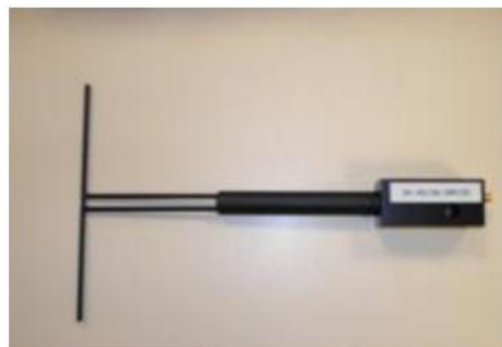
Figure 1 – Satimo COMOSAR Validation Dipole
