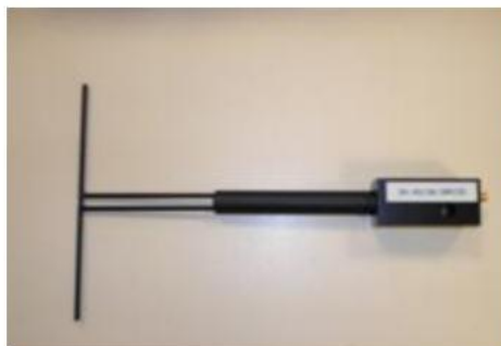
Figure 1 – Satimo COMOSAR Validation Dipole
