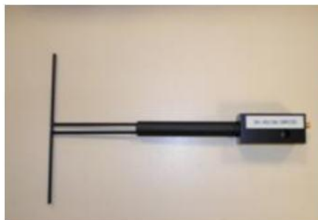
Figure 1 – Satimo COMOSAR Validation Dipole
