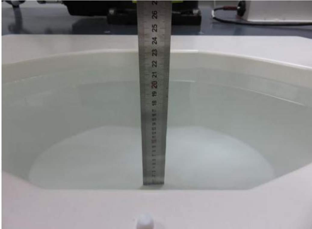
Photograph of the depth in the Head Phantom (5200MHz, 16.2cm depth)
