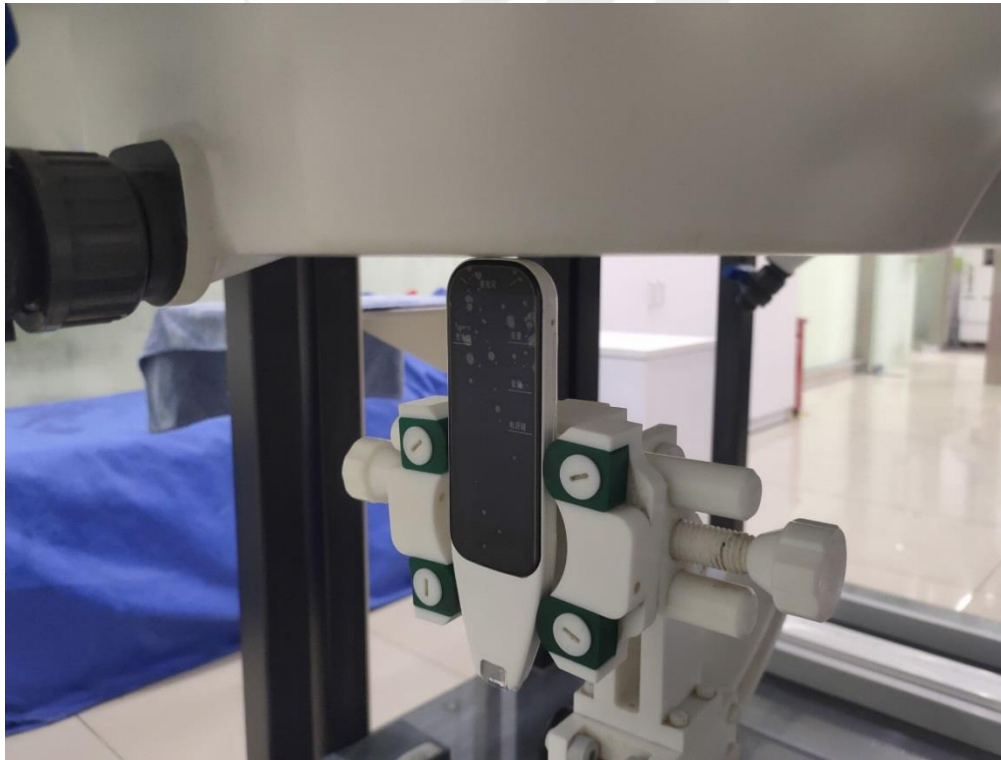
Body Top Edge (separation distance is 0mm)
