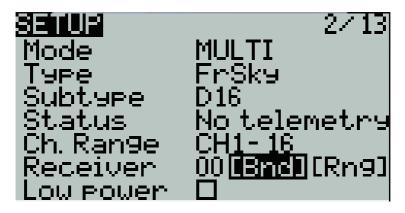
Long press the MDL button to enter the model settings, select MULTI in the SETUP page, and select the desired
