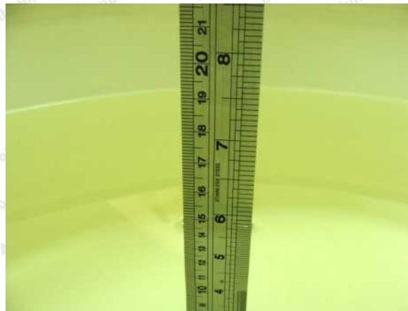
Photo of Liquid Height for Body SAR
