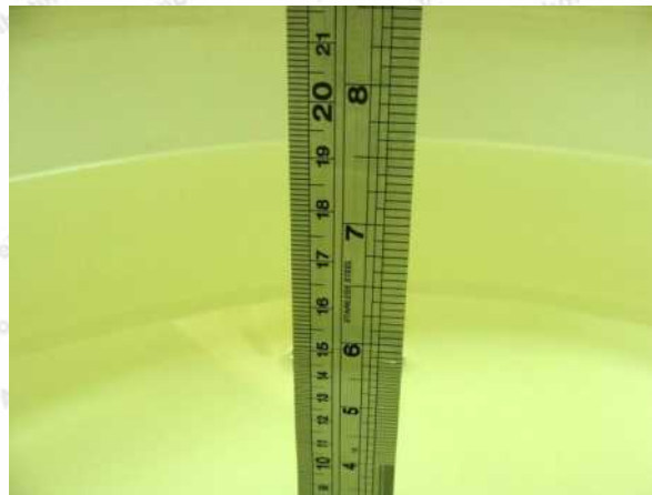
Photo of Liquid Height for Body SAR
