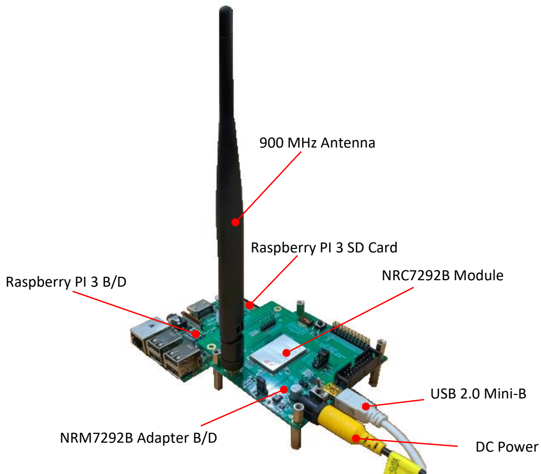
Figure 4.1 Antenna Connection on EVK
