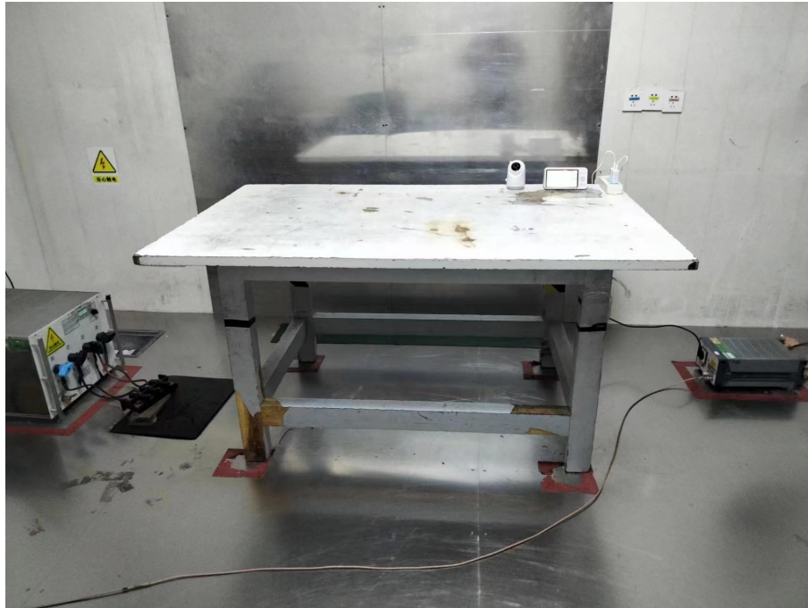
Photos of Conducted Emission Measurement
