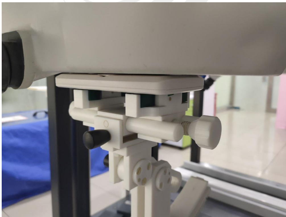
Body Back side(separation distance is 0mm)
