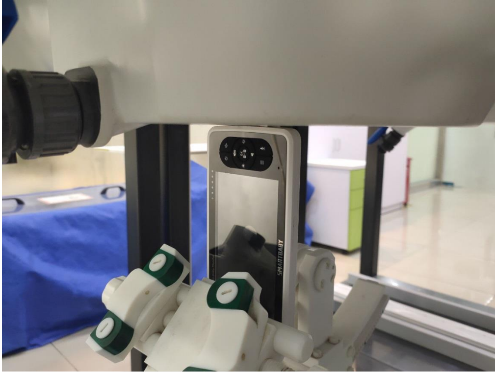
Body Right side(separation distance is 0mm)
