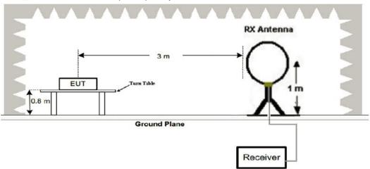
2. Radiated Emission Test-Up Frequency 30MHz~1GHz
